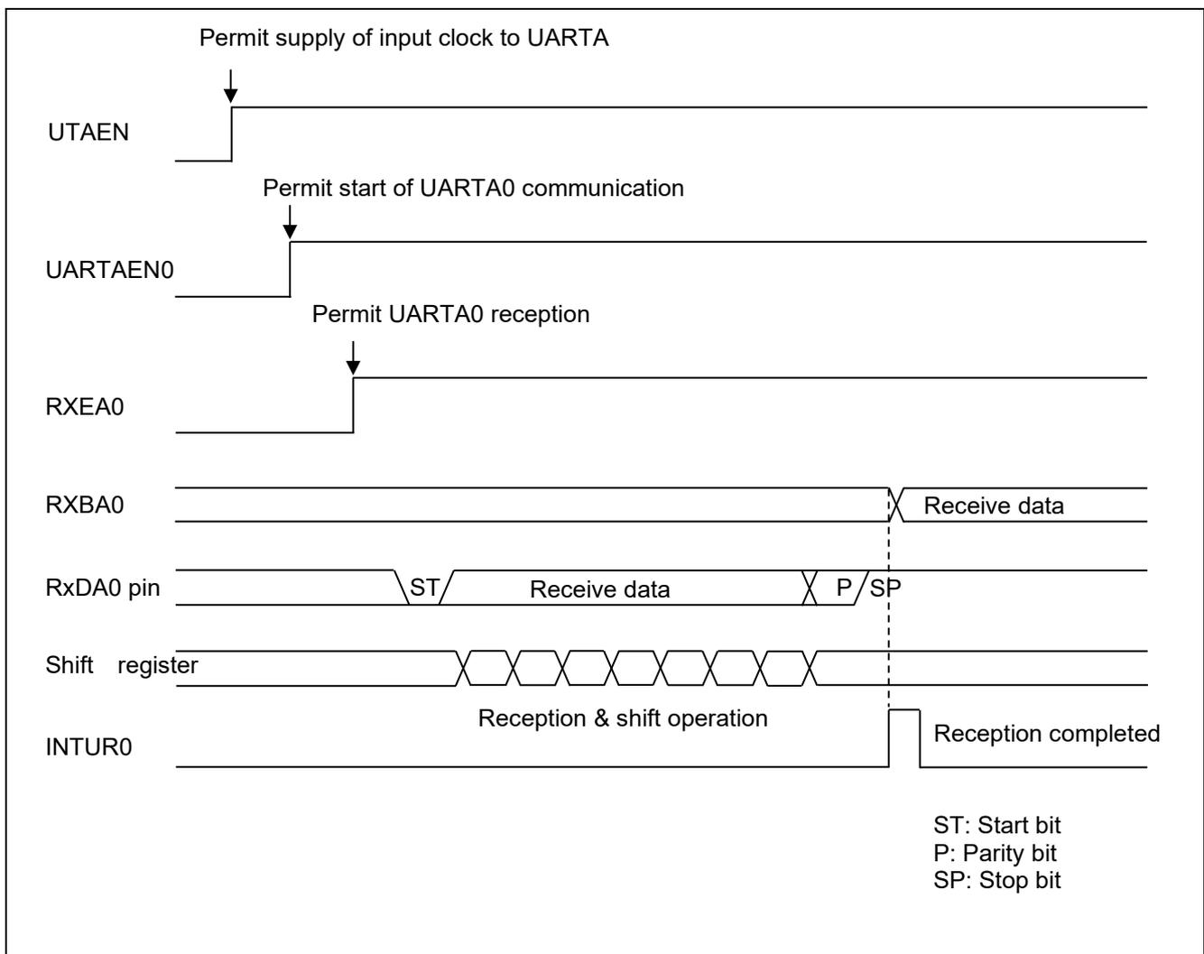
Figure 1.2 UART Transmission Timing Chart
