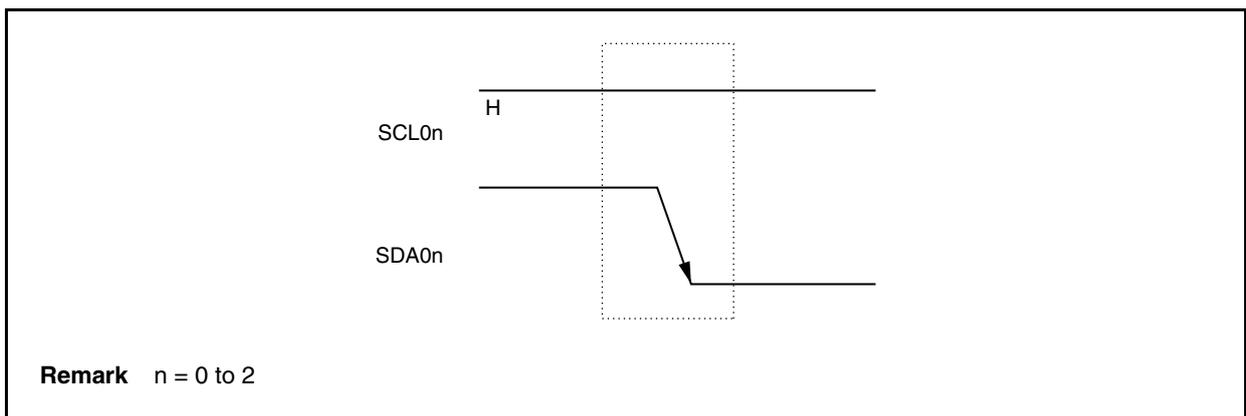
A start condition is generated when the IICn.STTn bit is set (1) after a stop condition has been detected (IICn.SPDn bit = 1). When a start condition is detected, the IICn.STDn bit is set (1) (n = 0 to 2).
