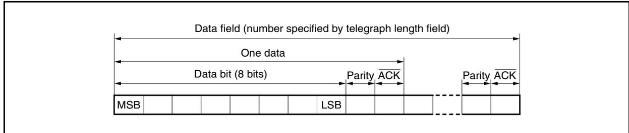
Following the data bit, the parity bit and acknowledge bit are respectively output by the master unit and slave unit.
