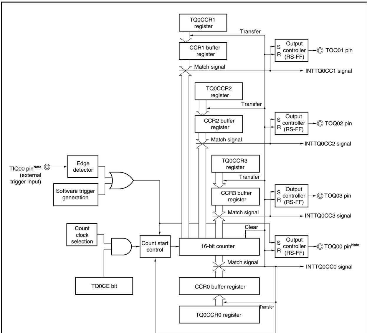
**Note** Because the external trigger input pin (TIQ00) and timer output pin (TOQ00) share the same alternate-function pin, two functions cannot be used at the same time.
