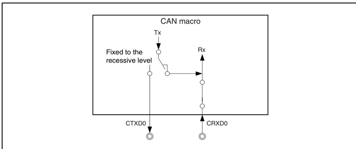
In the receive-only mode, no message frames can be transmitted from the CAN module to the CAN bus. Transmit requests issued for message buffers defined as transmit message buffers are held pending.
