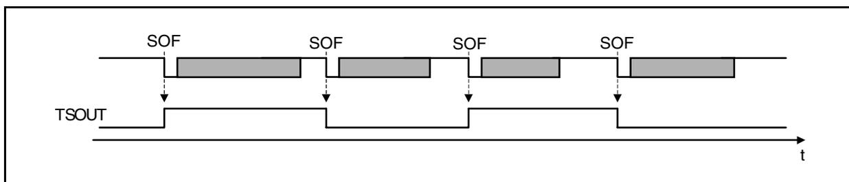
The TSOUT signal toggles its level upon occurrence of the selected event during data frame reception (in Figure 19-34, the SOF is used as the trigger event source). To capture a timer value by using the TSOUT signal, the capture timer unit must detect the capture signal at both the rising edge and falling edge.
