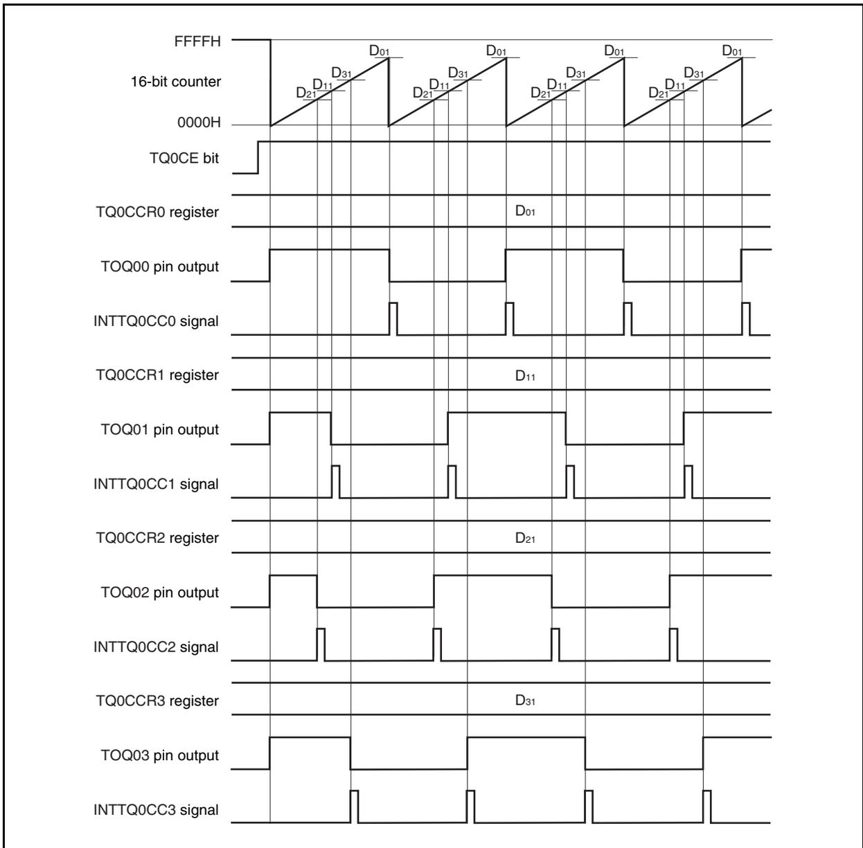
If the set value of the TQ0CCRk register is greater than the set value of the TQ0CCR0 register, the count value of the 16-bit counter does not match the value of the TQ0CCRk register. Consequently, the INTTQ0CCk signal is not generated, nor is the output of the TOQ0k pin changed. It is recommended to set the TQ0CCRk register to FFFFH when the TQ0CCRk register is not used.
