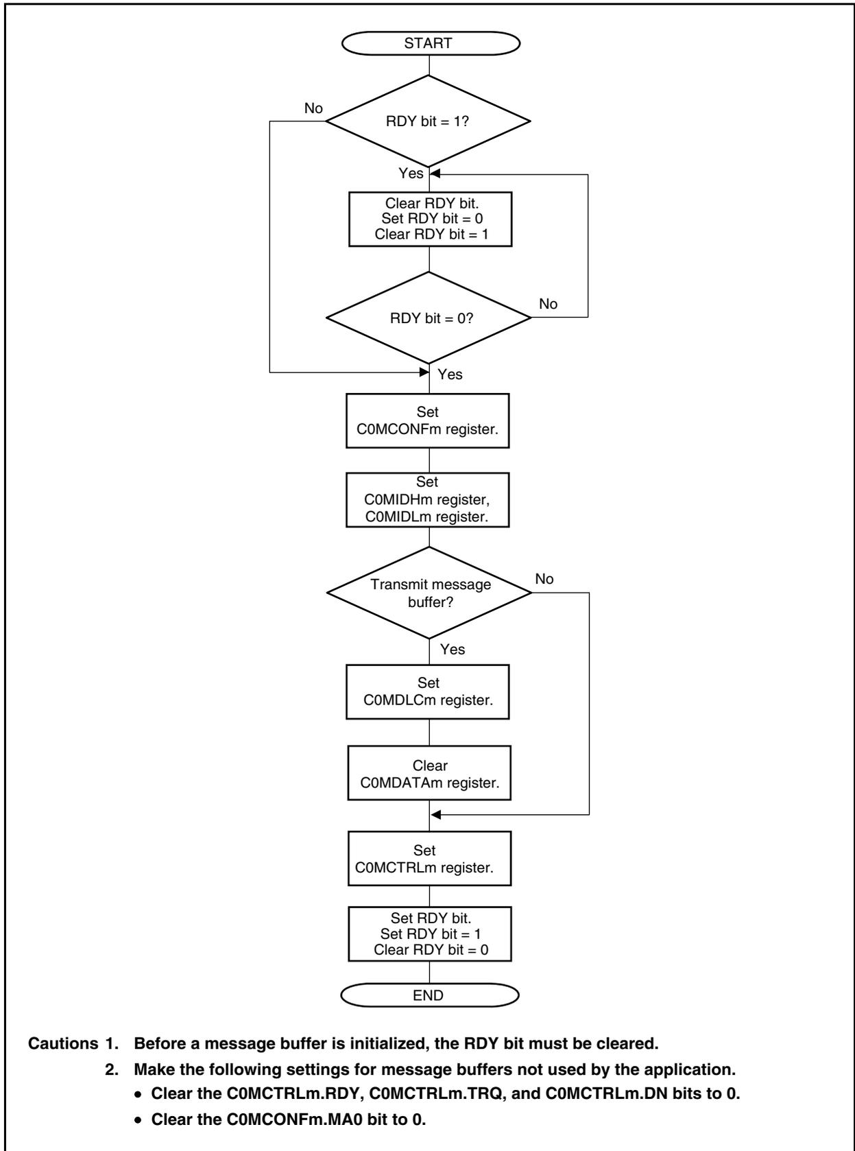
Figure 19-39 shows the processing for a receive message buffer (COMCONFm.MT2 to COMCONFm.MT0 bits = 001B to 101B).
