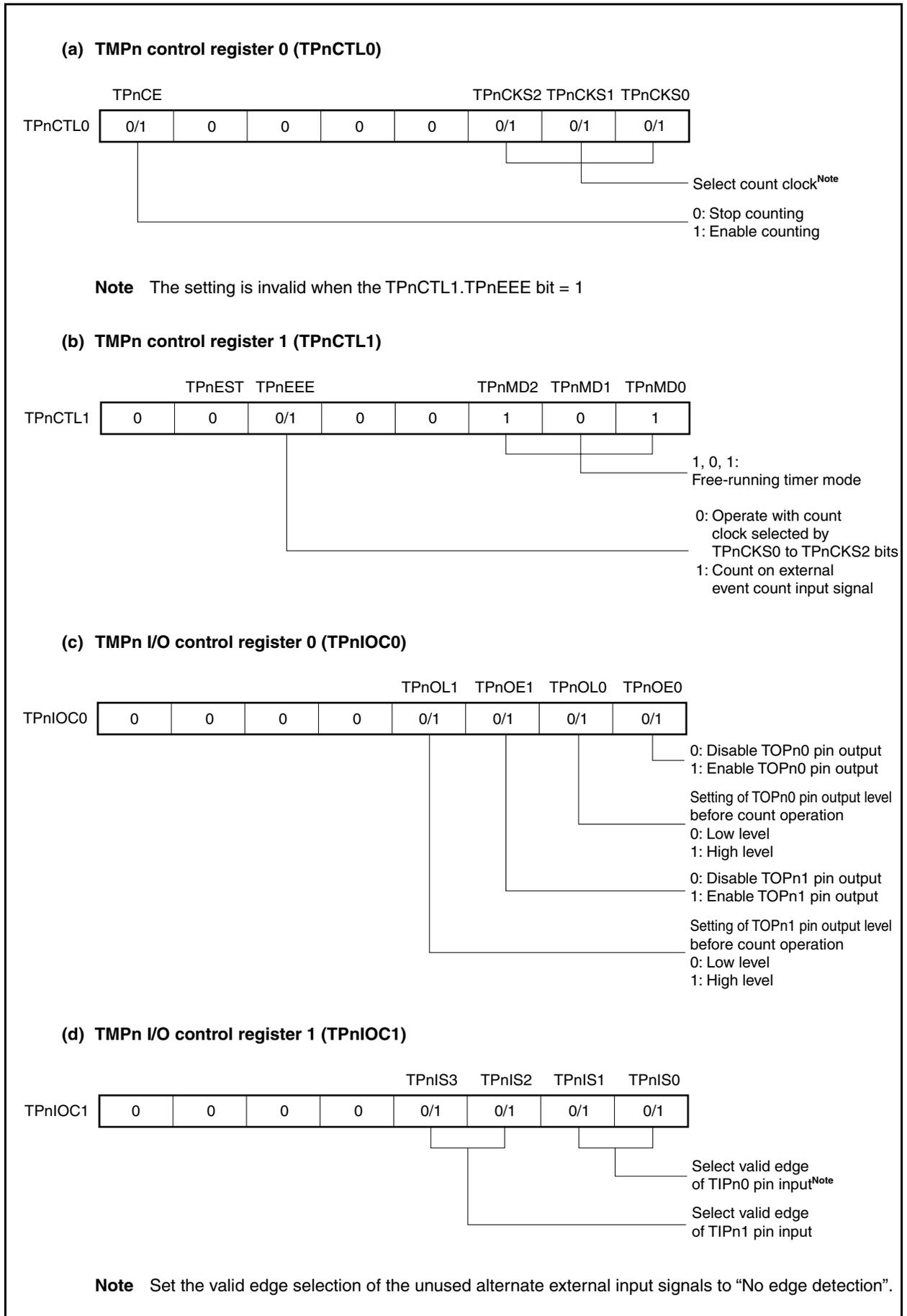
Figure 7-35. Register Setting in Free-Running Timer Mode (2/2)
