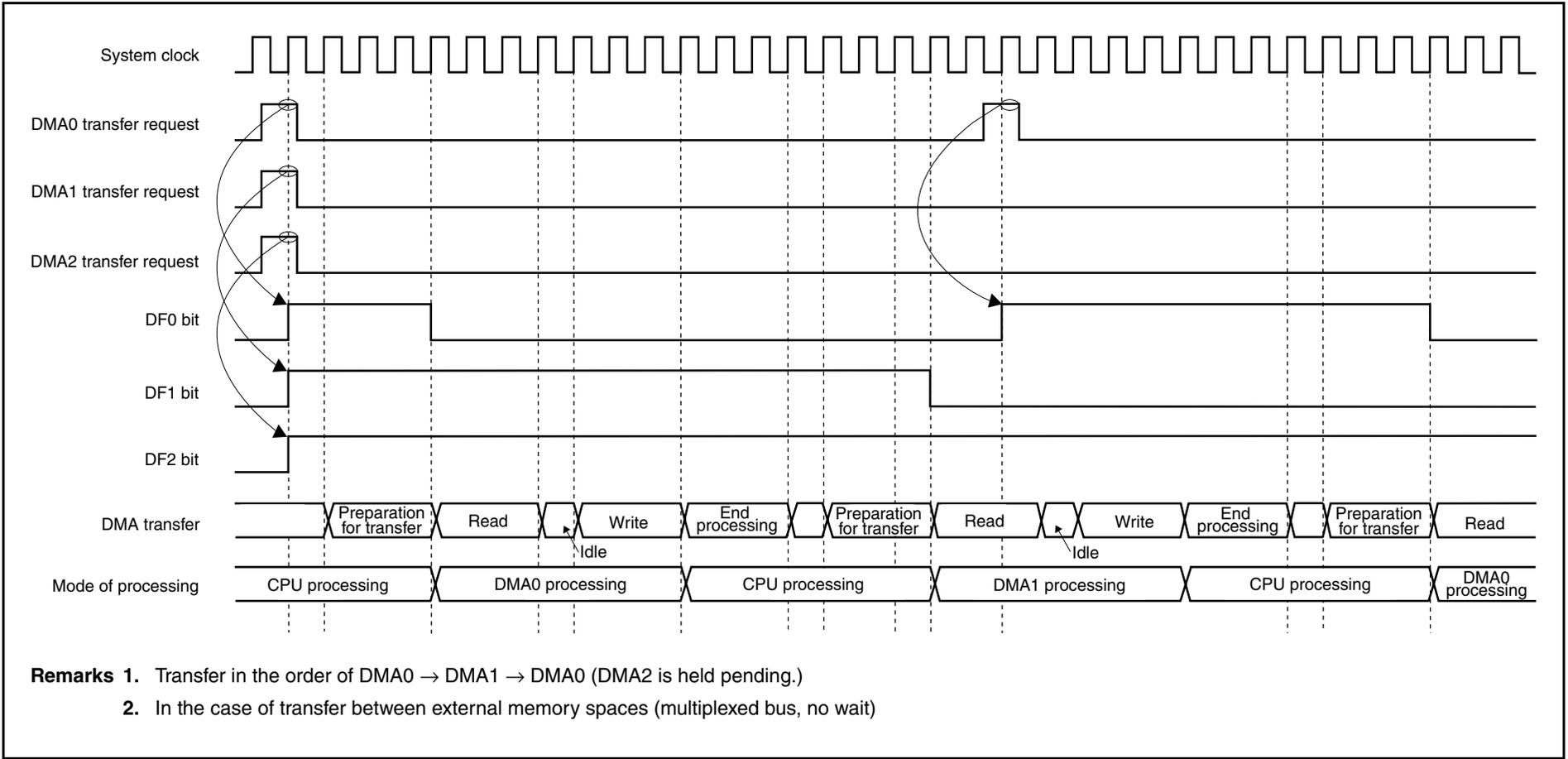
Figure 20-4. Period in Which DMA Transfer Request Is Ignored (1)
