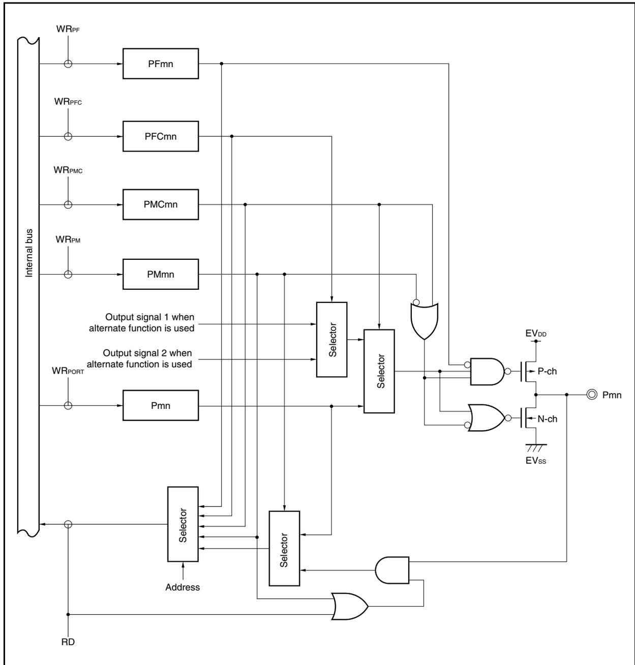
Figure 4-12. Block Diagram of Type G-4
