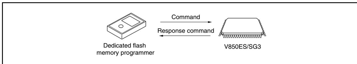
The following shows the commands for flash memory control in the V850ES/SG3. All of these commands are issued from the dedicated flash memory programmer, and the V850ES/SG3 performs the processing corresponding to the commands.
