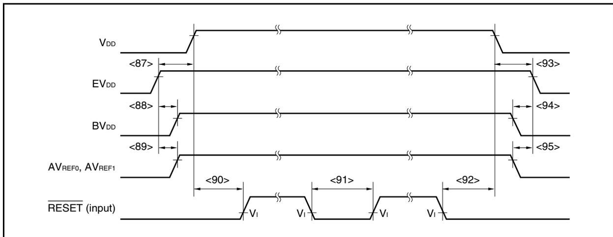
**(2) Interrupt, FLMD0 Pin Timing****(T<sub>A</sub> = -40 to +85°C, BV<sub>DD</sub> ≤ V<sub>DD</sub> = EV<sub>DD</sub> = AV<sub>REF0</sub> = AV<sub>REF1</sub>, V<sub>SS</sub> = EV<sub>SS</sub> = BV<sub>SS</sub> = AV<sub>SS</sub> = 0 V, C<sub>L</sub> = 50 pF)**
