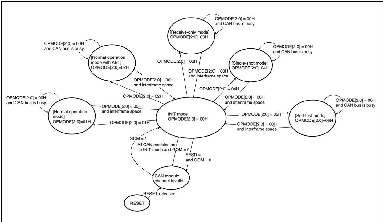
The transition from the initialization mode to an operation mode is controlled by the C0CTRL.OPMODE2 to C0CTRL.OPMODE0 bits.
