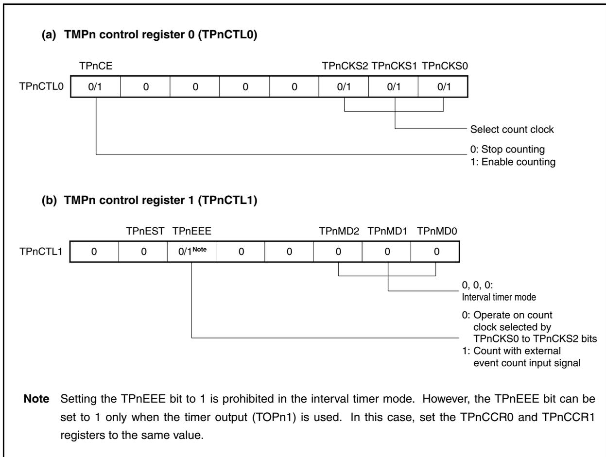
Figure 7-8. Register Setting for Interval Timer Mode Operation (2/2)
