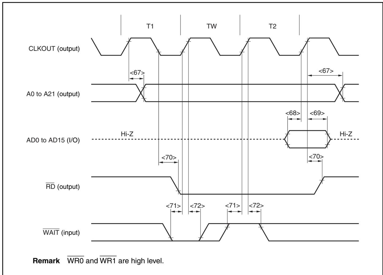
**(d) Write cycle (CLKOUT synchronous): In separate bus mode****( $T_A = -40$  to  $+85^\circ\text{C}$ ,  $BV_{DD} \leq V_{DD} = EV_{DD} = AV_{REF0} = AV_{REF1}$ ,  $V_{SS} = EV_{SS} = BV_{SS} = AV_{SS} = 0$  V,  $C_L = 50$  pF)**
