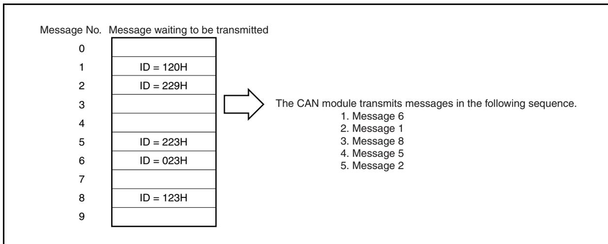
After the transmit message search, the transmit message with the highest priority of the transmit message buffers that have a pending transmission request (message buffers with the TRQ bit set to 1 in advance) is transmitted.
