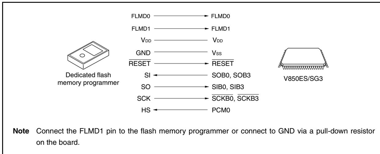
The dedicated flash memory programmer outputs the transfer clock, and the V850ES/SG3 operates as a slave.
