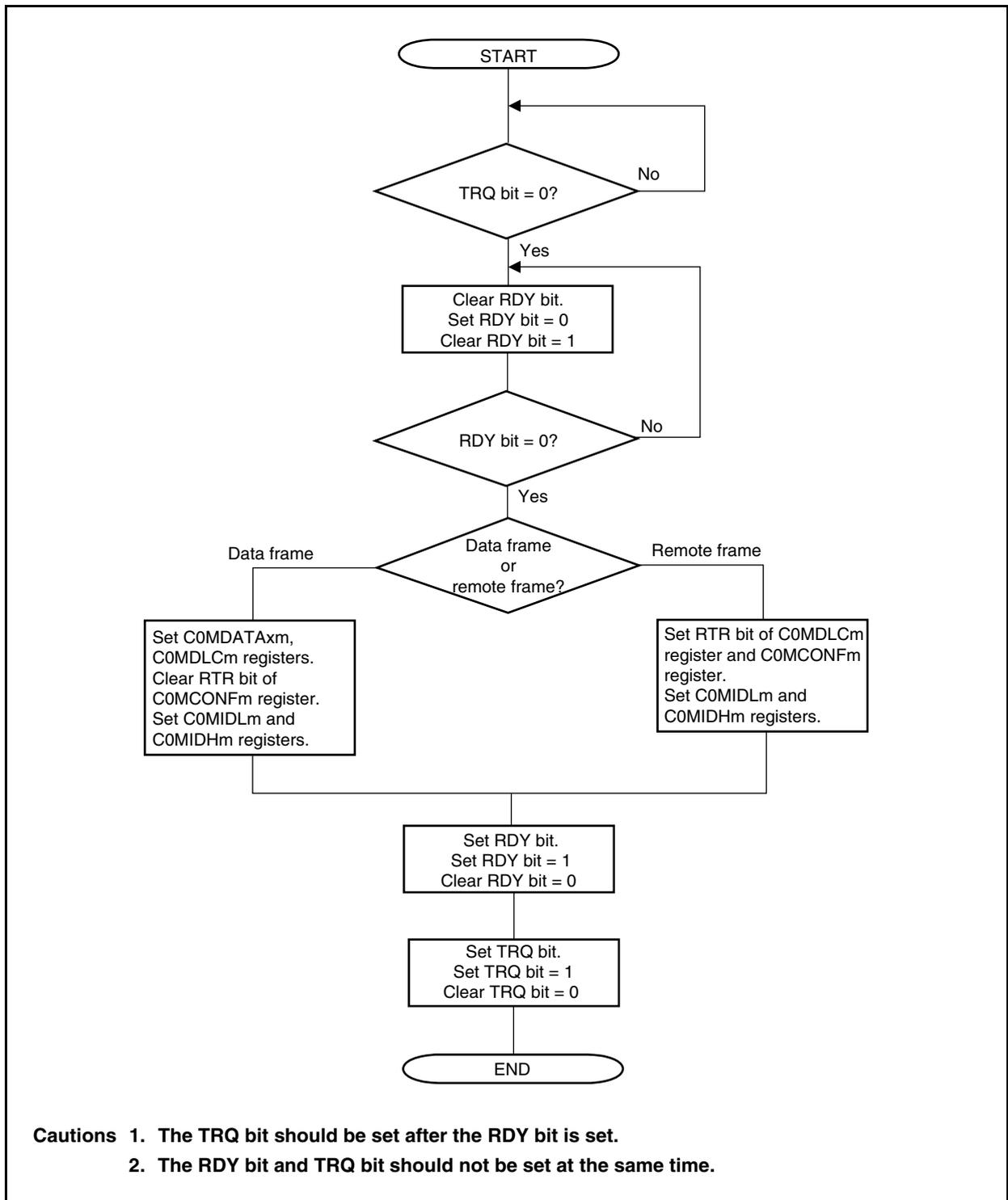
Figure 19-42 shows the processing for a transmit message buffer (COMCONFm.MT2 to COMCONFm.MT0 bits = 000B).
