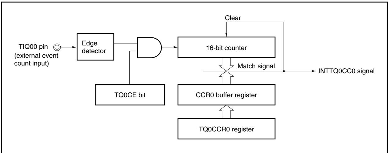
**Figure 8-14. Basic Timing in External Event Count Mode**
