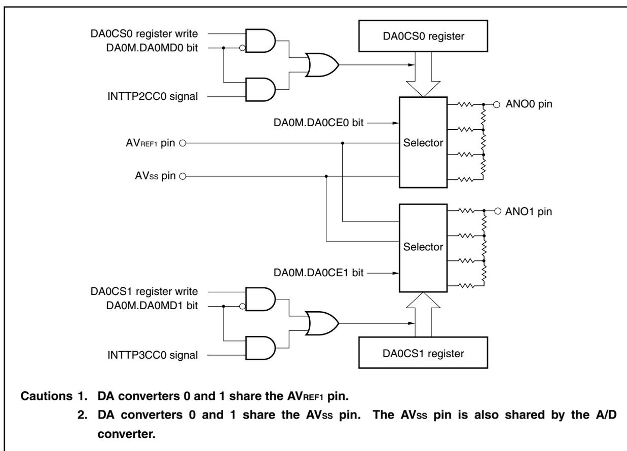
The D/A converter includes the following hardware.
