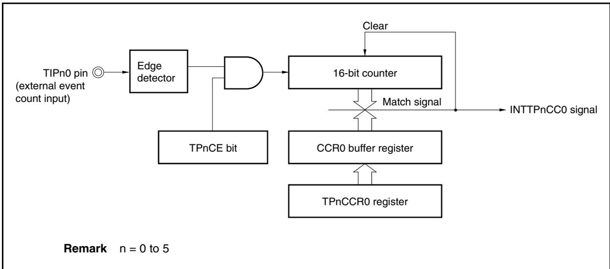
**Figure 7-14. Basic Timing in External Event Count Mode**
