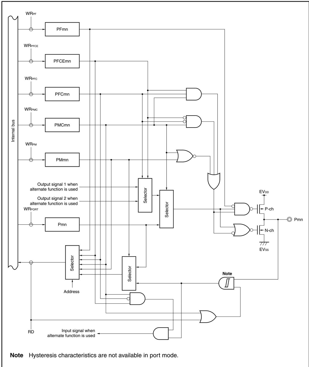
Figure 4-31. Block Diagram of Type U-15
