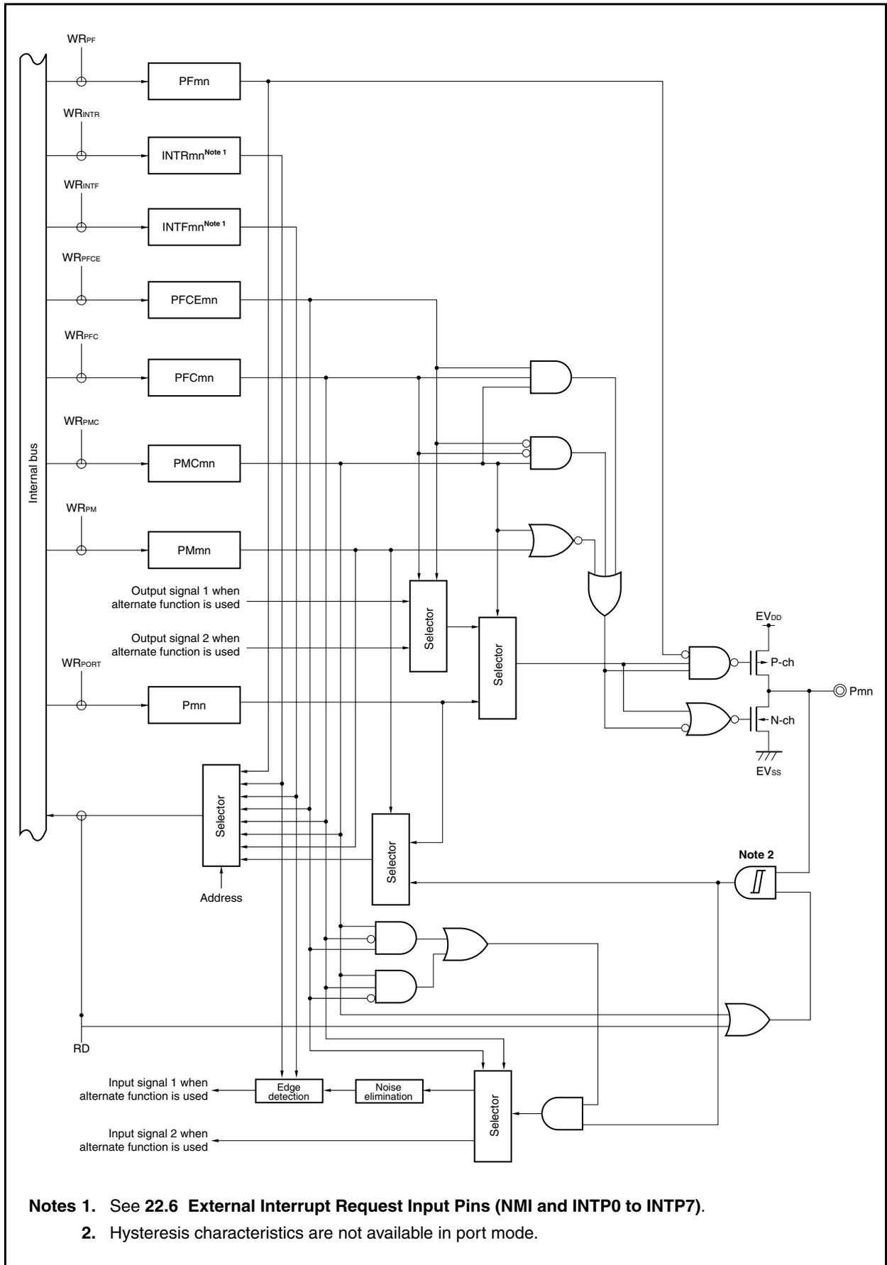
Figure 4-32. Block Diagram of Type AA-1
