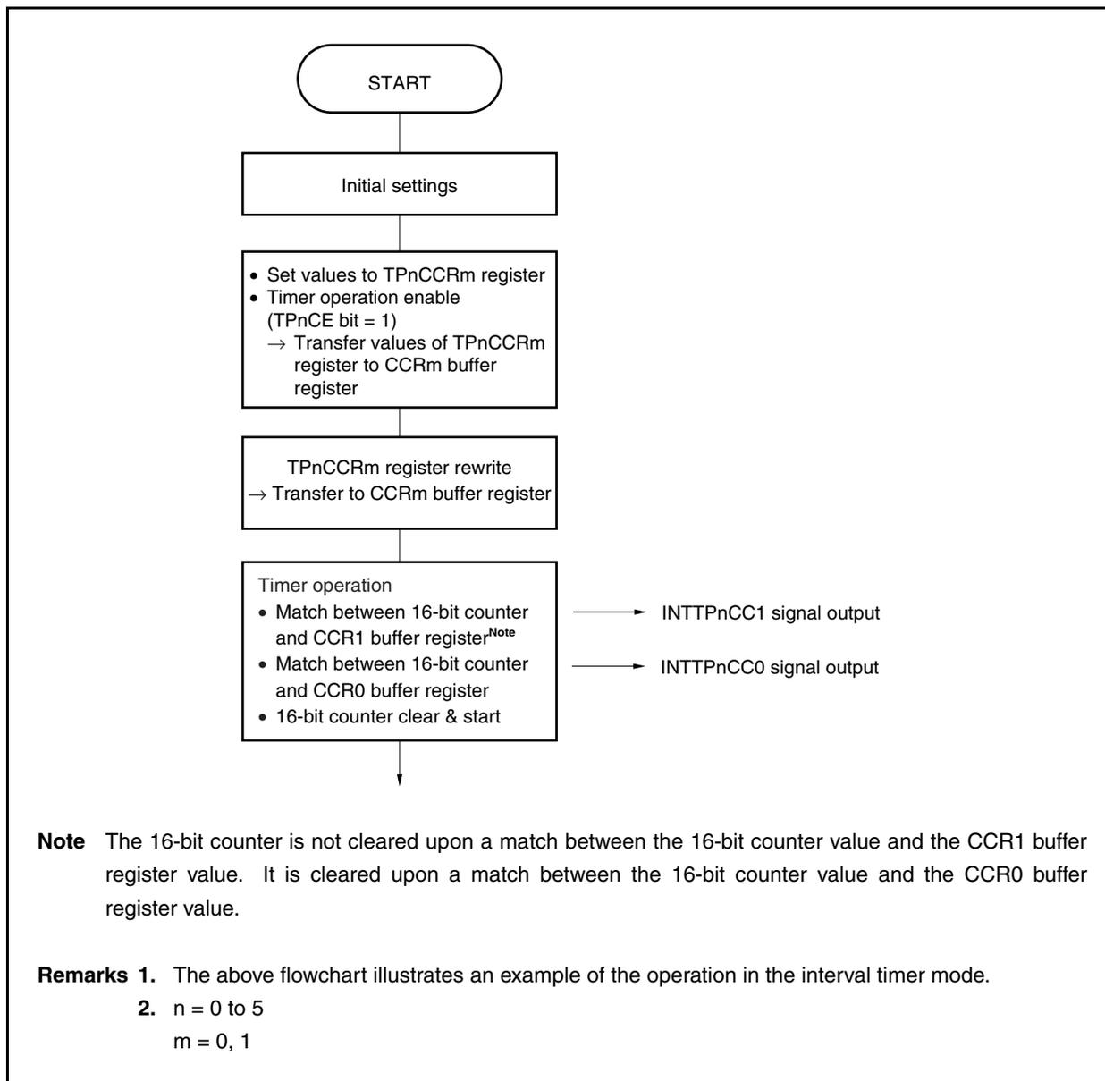
Figure 7-3. Timing of Anytime Write
