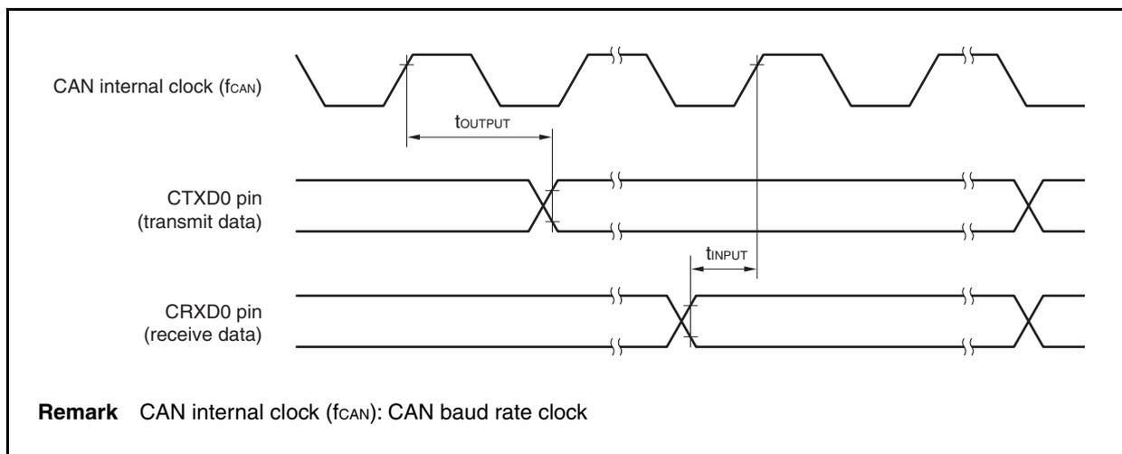
Internal delay time ( $t_{NODE}$ ) = Internal transmission delay time ( $t_{OUTPUT}$ ) + Internal reception delay time ( $t_{INPUT}$ )
