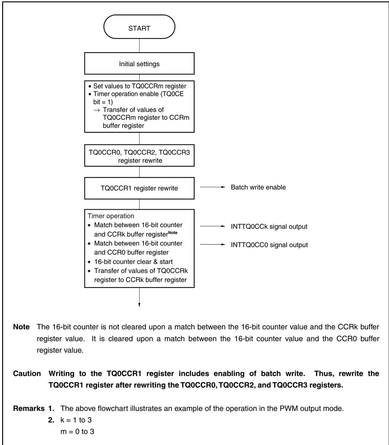
Figure 8-5. Timing of Batch Write
