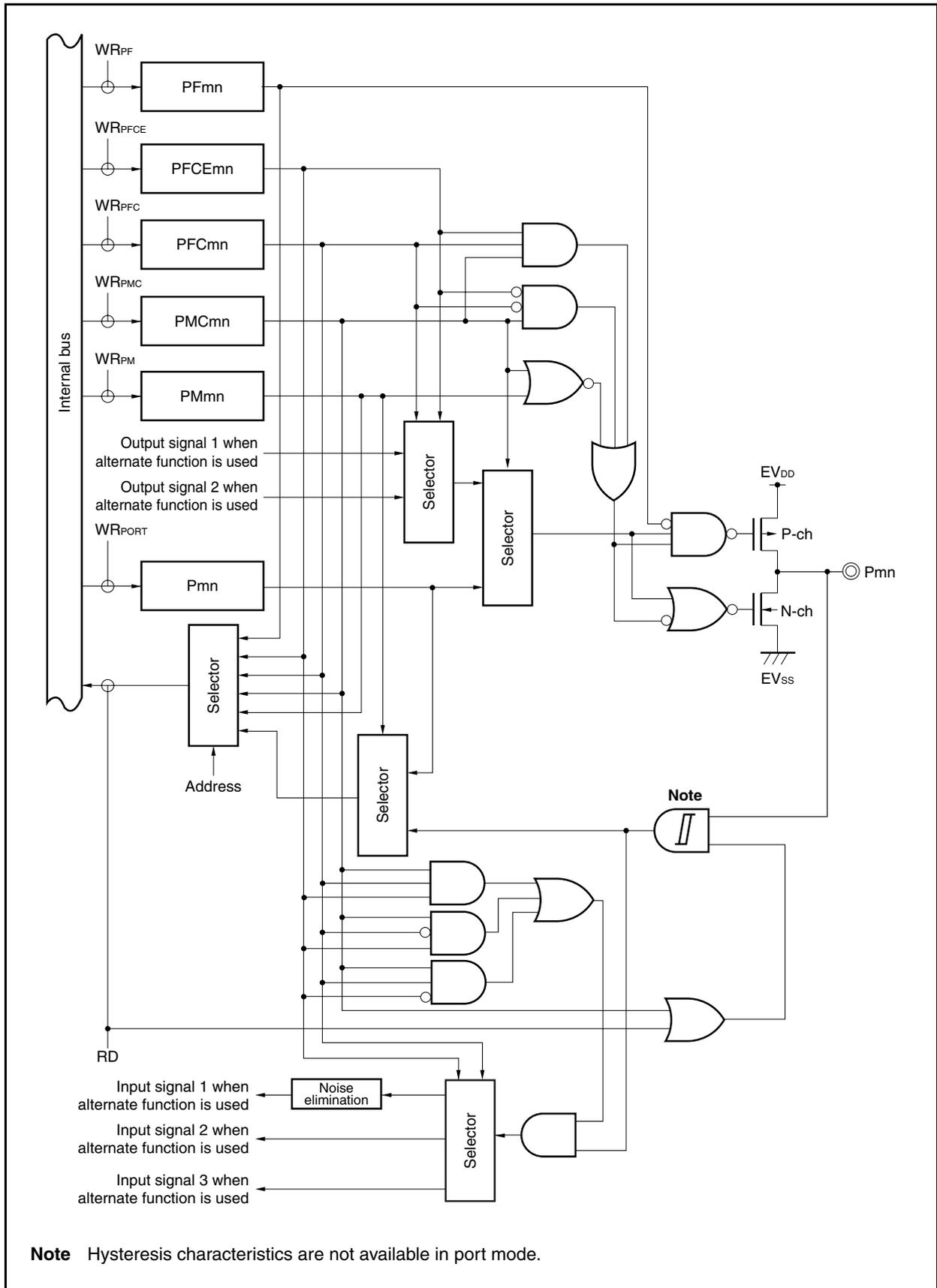
Figure 4-28. Block Diagram of Type U-12
