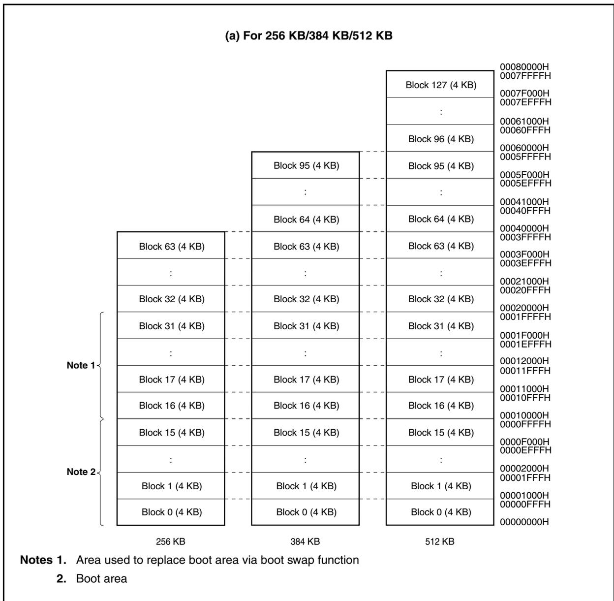
Figure 30-1. Flash Memory Mapping (2/2)
