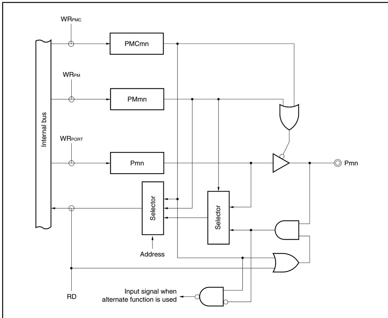
Figure 4-7. Block Diagram of Type D-3
