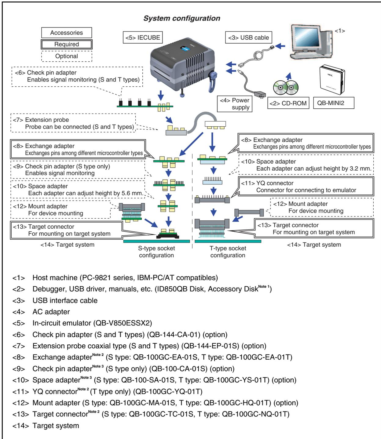
**Figure A-3. System Configuration (QB-V850ESSX2 Used) (2/2)**
