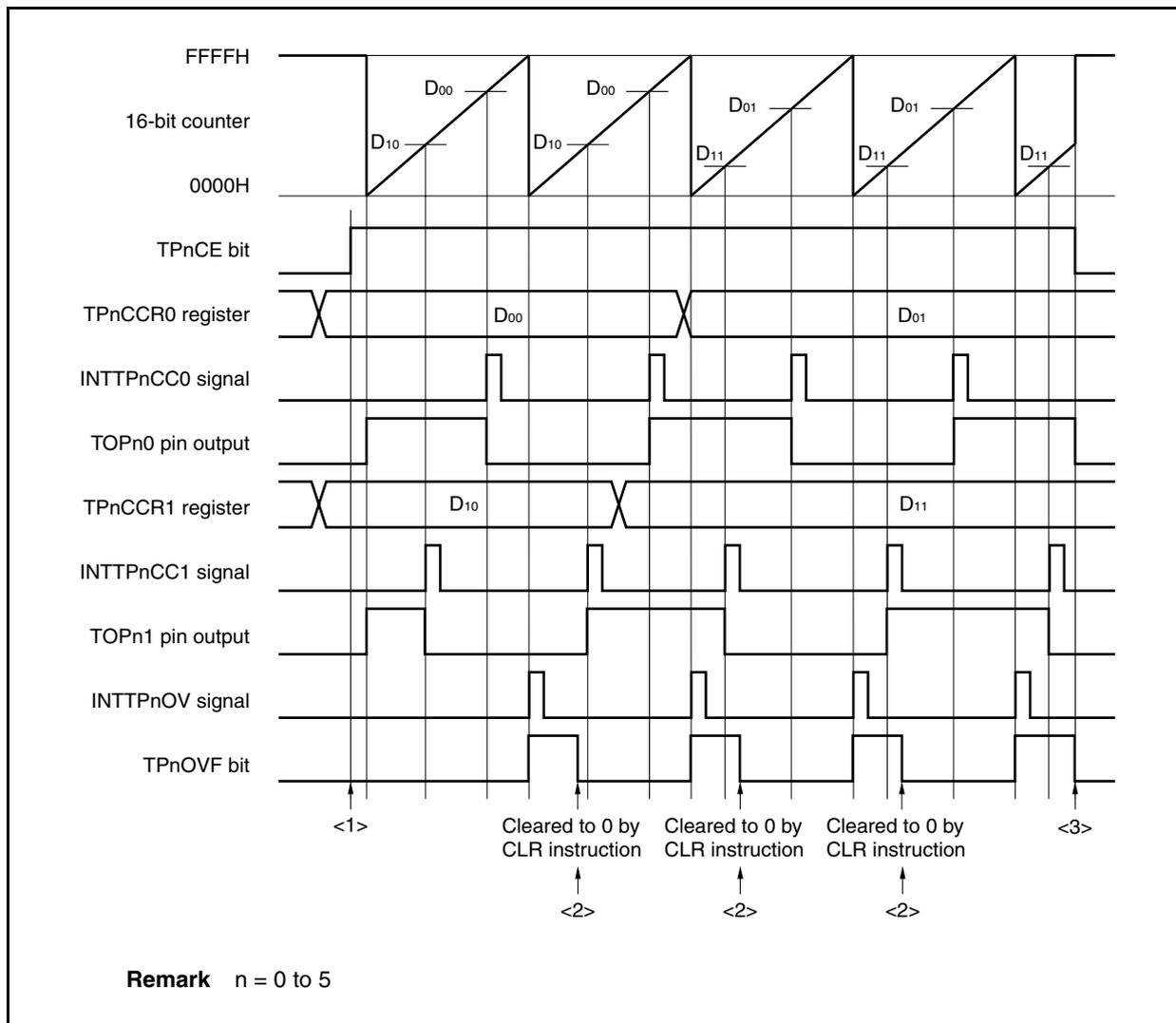
Figure 7-36. Software Processing Flow in Free-Running Timer Mode (Compare Function) (2/2)
