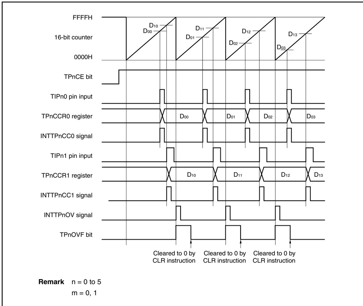
Figure 7-35. Register Setting in Free-Running Timer Mode (1/2)
