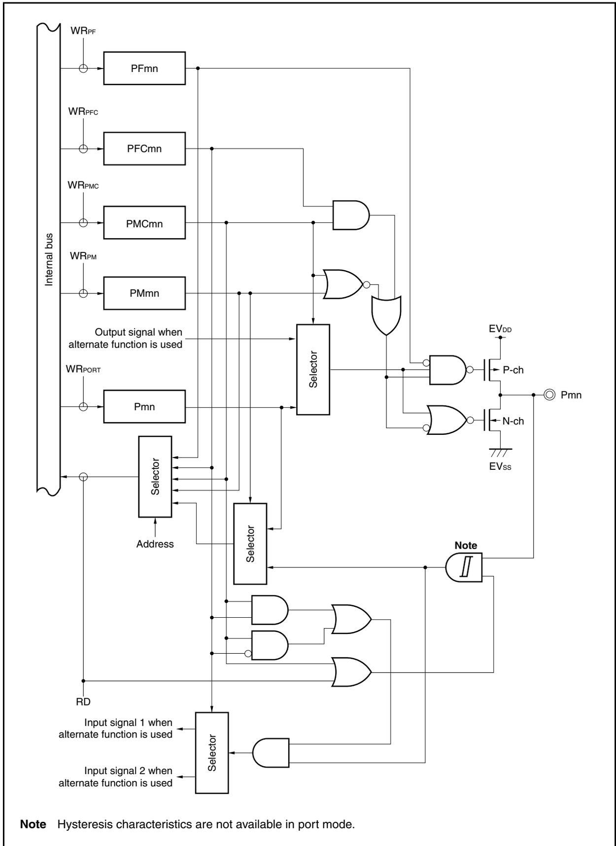
Figure 4-15. Block Diagram of Type G-12
