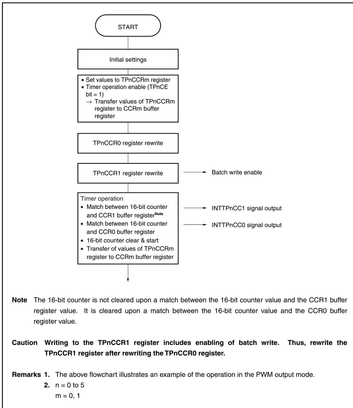
Figure 7-5. Timing of Batch Write
