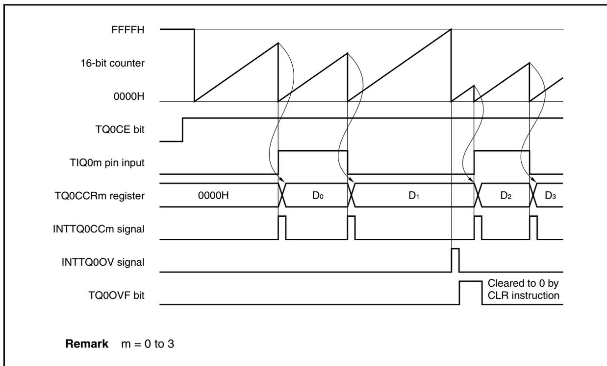
When the TQ0CE bit is set to 1, the 16-bit counter starts counting. When the valid edge input to the TIQ0m pin is later detected, the count value of the 16-bit counter is stored in the TQ0CCRm register, the 16-bit counter is cleared to 0000H, and a capture interrupt request signal (INTTQ0CCm) is generated.
