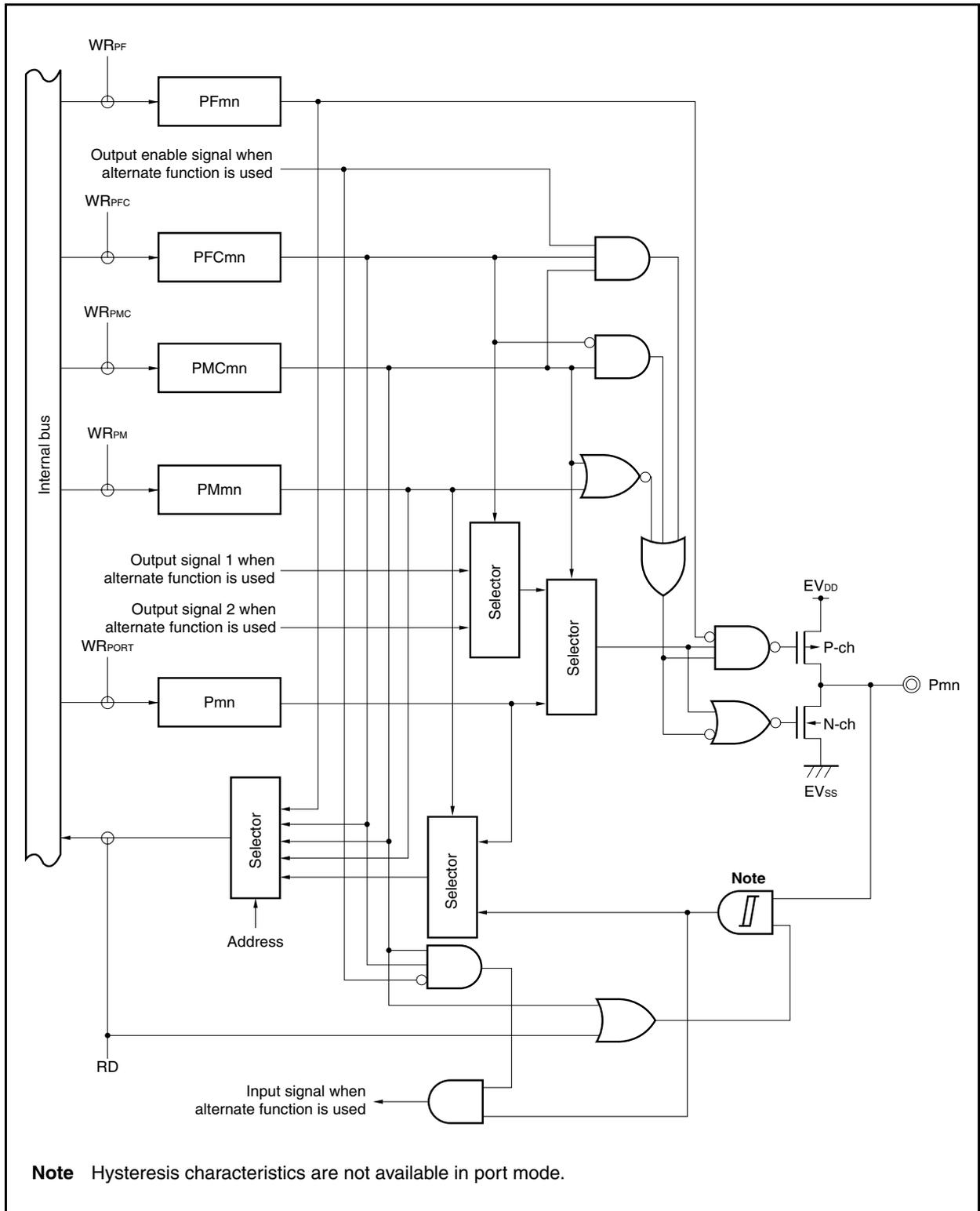
Figure 4-14. Block Diagram of Type G-6
