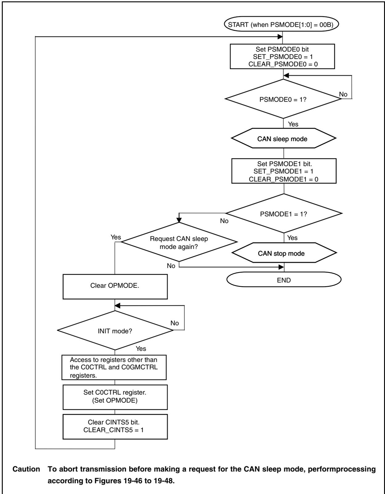
**Caution** To abort transmission before making a request for the CAN sleep mode, perform processing according to Figures 19-46 to 19-48.
