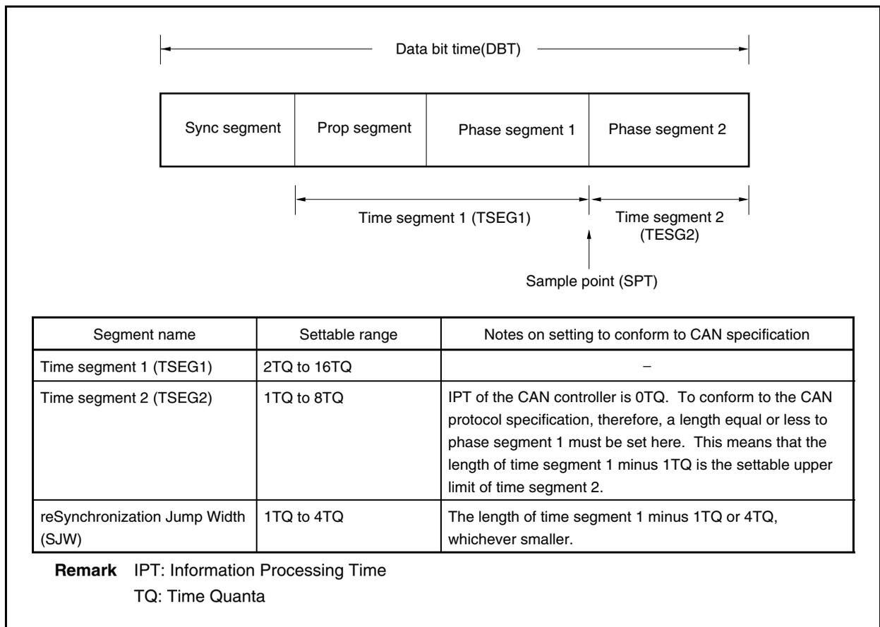
**Remark** The CAN protocol specification defines the segments constituting the data bit time as shown in Figure 19-19.
