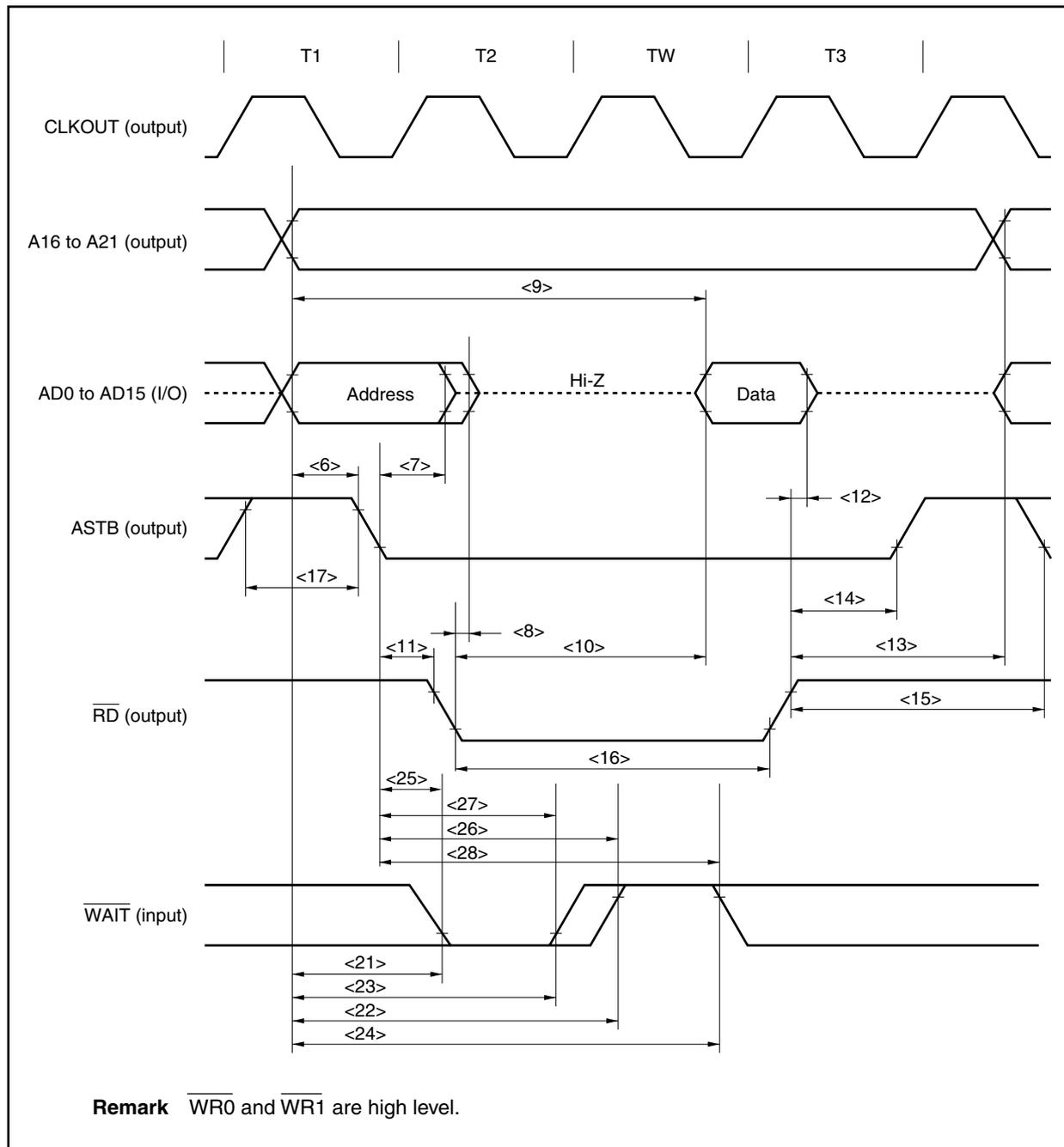
**Write Cycle (CLKOUT Asynchronous): In Multiplexed Bus Mode**
