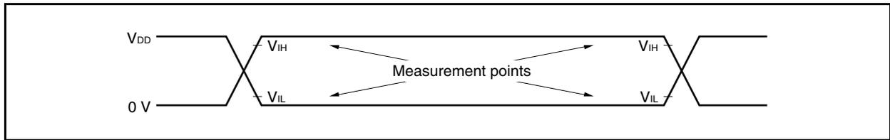
(2) AC Test Output Measurement Points
