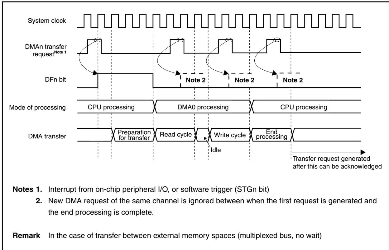
Figure 20-5. Period in Which DMA Transfer Request Is Ignored (2)
