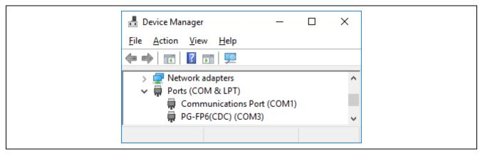
Figure 7.1 Checking the COM Port Number Settings
