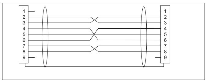
Figure 10.5 Connection of the Serial Cable
