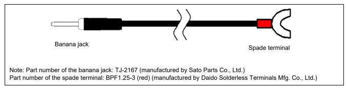
Figure 10.14 Appearance of the GND Cable
