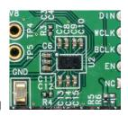
The SmartBeat<sup>™</sup> DA7402 is a high-performance, ultra-low-power stereo hi-fi codec. Featuring Dialog's custom digital hybrid ANC technology, it offers stronger suppression of ambient noise over a wider range of frequencies for the best user experience in any environment.
