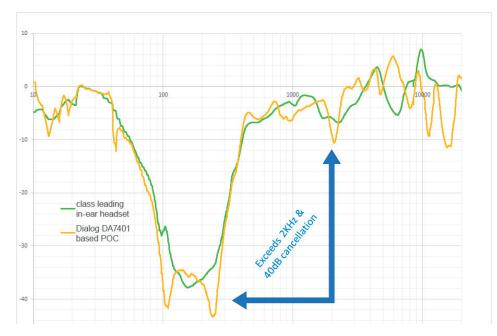
Key to this performance is a custom DSP that is optimized for ANC and enables an input-to-output latency of just 25 µs. Meanwhile a dedicated fast equalization (FEQ) path operating at the digital microphone (DMIC) clock rate improves cancellation at high frequencies.
