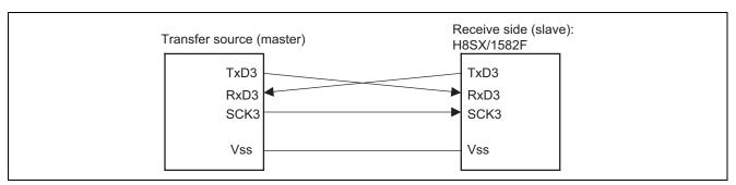
Figure 2 Wiring for Clock Synchronous Communications
