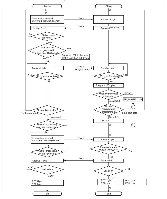
Figure 12 Programming Processing
