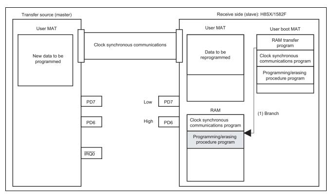
Figure 7 Activation of Programming/Erasing Procedure Program
