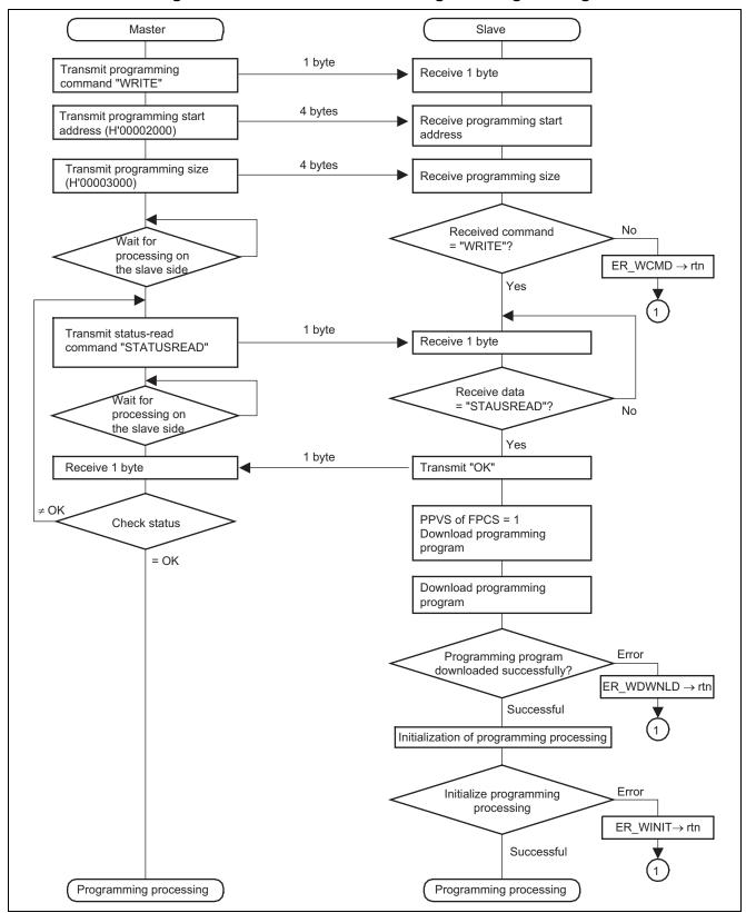
Figure 11 Processing to Receive the Position and Range for Programming
