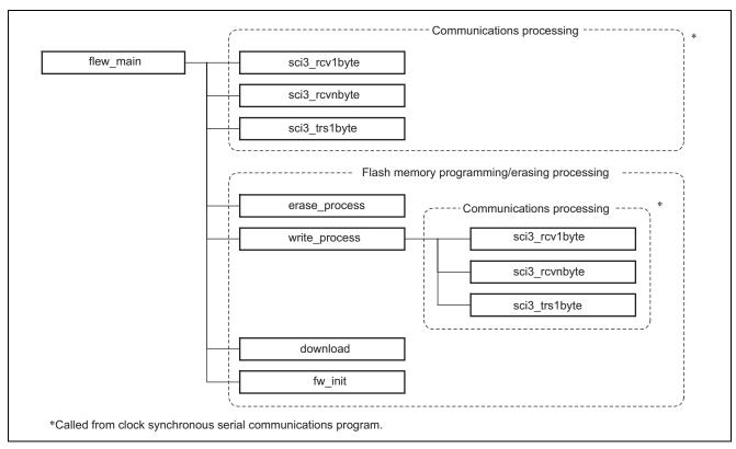
Figure 14 Programming/Erasing Procedure Program
