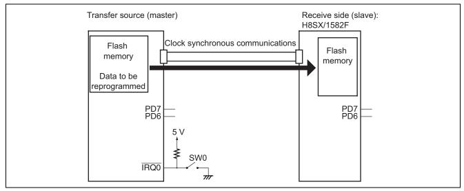
Figure 1 Sample Configuration for On-Board Reprogramming
