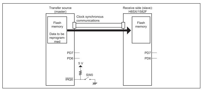
Figure 1 Sample Configuration for On-Board Reprogramming
