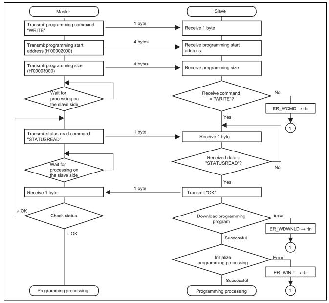
Figure 15 Processing to Receive the Position and Range for Programming
