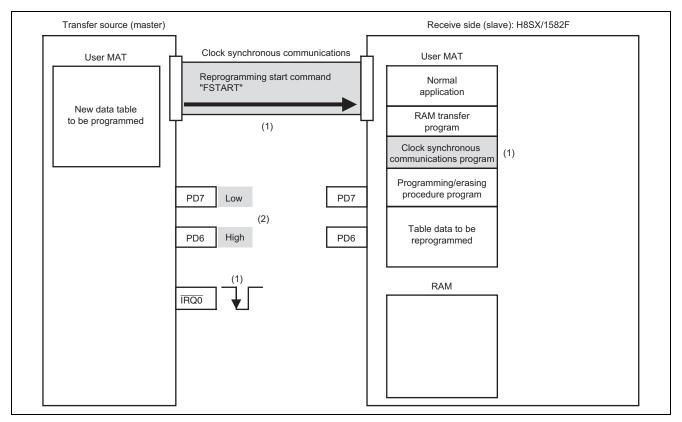
Figure 7 Preparation of On-Board Reprogramming
