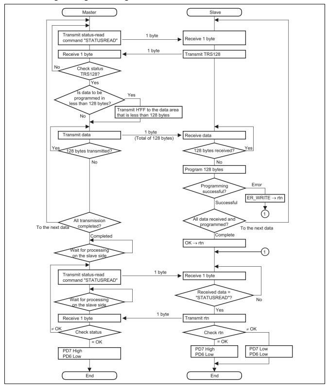
Figure 16 Programming Processing
