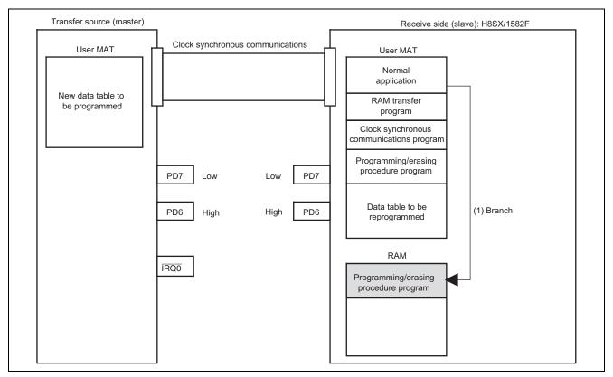
Figure 9 Activation of Programming/Erasing Procedure Program
