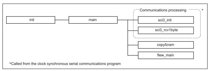
Figure 17 Normal Program on the Slave Side
