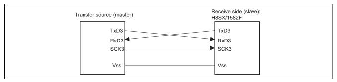
Figure 2 Wiring for Clock Synchronous Communications
