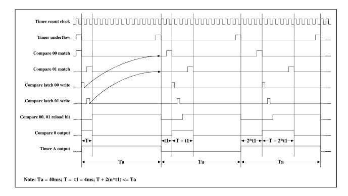
Fig.1: The Operate Timing and Output Waveform of Output Compare Mode
