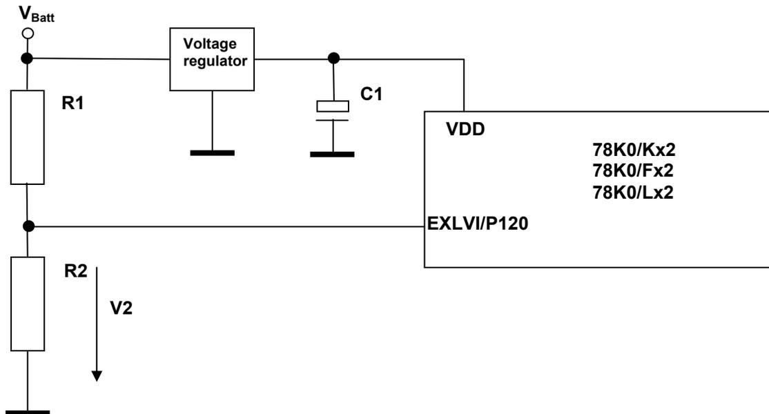
Normal operation:  $V2 = V_{Batt} \times R2 / (R1 + R2) > 1.31V$
