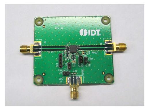
Figure 2. TRL Calibration Board used for the F0480
