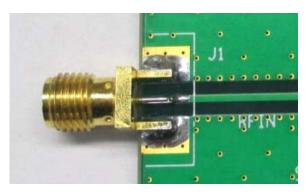
The advantage of performing time domain analysis is that response can be gated so that the response of only the particular time window selected is examined. This is done by setting the magnitude to zero, no discontinuity. Since we want to examine what the input connector and board connection is doing, we can gate the time domain response window from -0.2 to 0.2 ns. All other time is forced to zero. Because this is the first component in the circuit, masking concerns are not needed.
