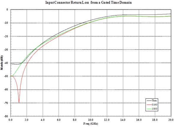
The input match is only for the connector and board connection. Using the gated response removed the resonance with the
