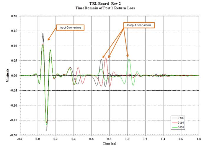
Figure 4 shows where the discontinuities lie while using a Low pass response time domain analysis. The first discontinuity is the input connector and connection to the evaluation board. Though there are slight magnitude differences, note that the shape and position are exact. This shows that the three different connectors all very similar. The output connect can be seen between 0.7 and 1.0 ns. The magnitude is less than the input connector because of masking.
