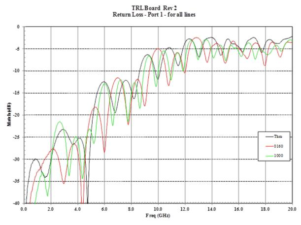
Notice the high ripple content and the variance depending on the length of line. This is due to the mismatch of connectors resonating. Transforming to the time domain shows where the discontinuities are located.
