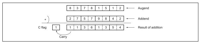
Figure 2 Example of Addition with a Carry
