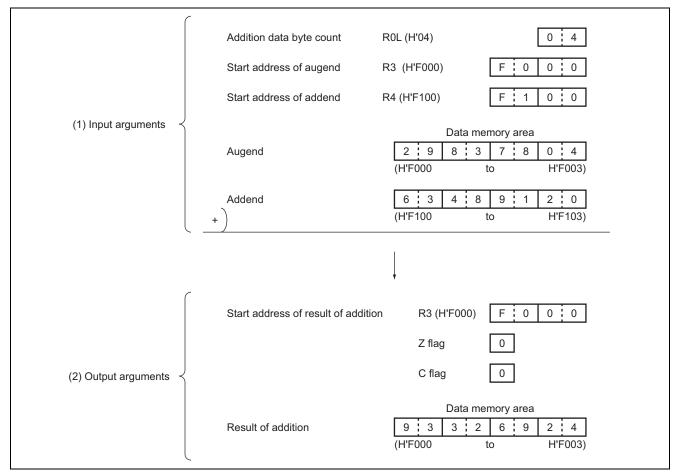
Figure 1 Example of Software ADDD2 Execution
