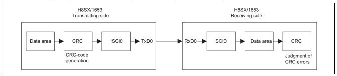
Figure 1 Asynchronous Transfer of Data with Appended CRC Codes via an SCI
