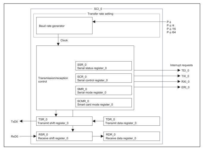
Figure 2 Block Diagram of SCI\_0
