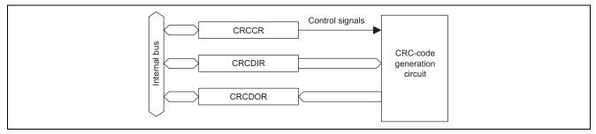
Figure 3 Block Diagram of the CRC Calculator
