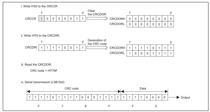
Figure 4 LSB-First Data Transmission
