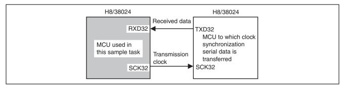
Figure 1 Clock Synchronization Serial Data Master Reception with the H8/38024
