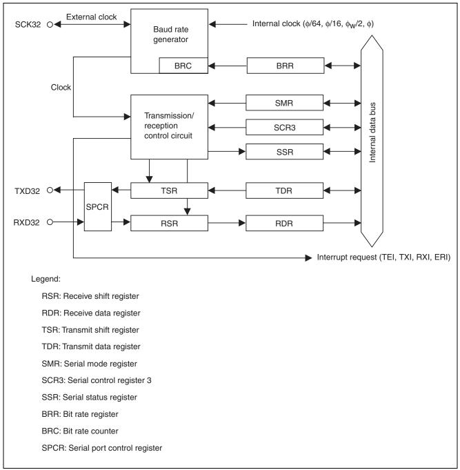
Figure 2 Block Diagram of SCI3
