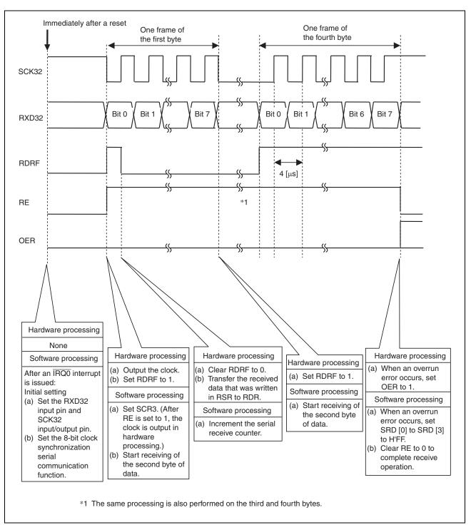
Figure 3 Operation during Reception of Data
