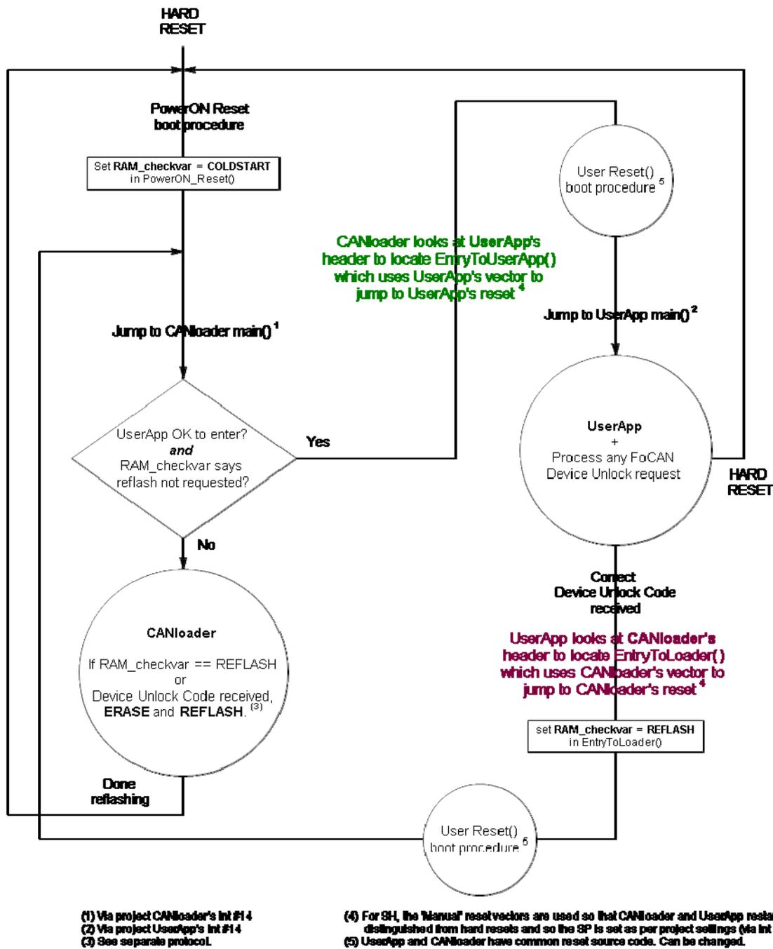
Figure 7. For SH devices the FoCAN boot and handover procedure between CANloader and UserApp is slightly different from the R8C/M16C/R32C family C-startup in that the Manual reset vector is used when the projects transfer control to each other.
