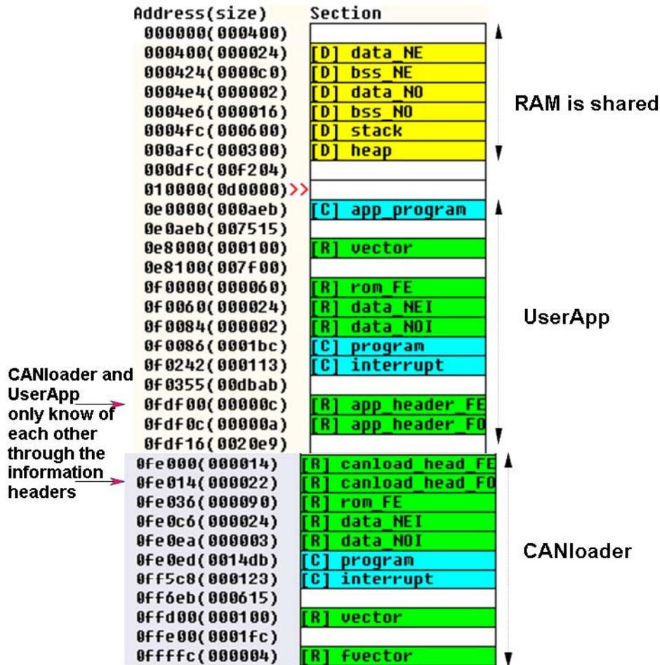
Figure 5 For R8C, M16C and R32C block zero is at the high end of the address spectrum. Note the red arrows indicating headers. This example shows an M16C/6Nx MCU.
