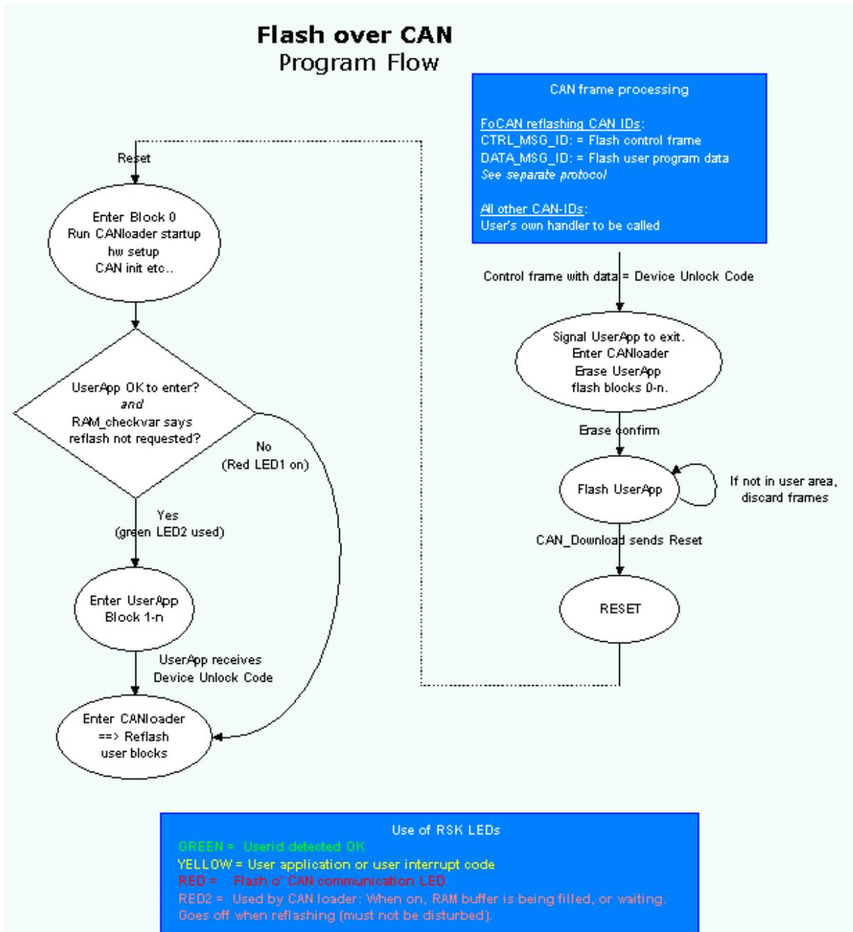
Figure 2. Program flow. To the left: Reset, CANloader’s startup code, and entering the user application (UserApp). To the right is shown processing of CAN frames in UserApp and in turn CANloader if a valid download is asserted.
