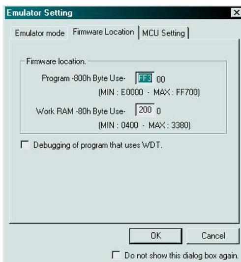
**Figure 8.** You can place the target debug kernel code in block 0 above canloader at a higher address and thereby leave all of UserApp free for your code. See the map file of your CANloader project to find free space in block 0 that the debugger can use.
