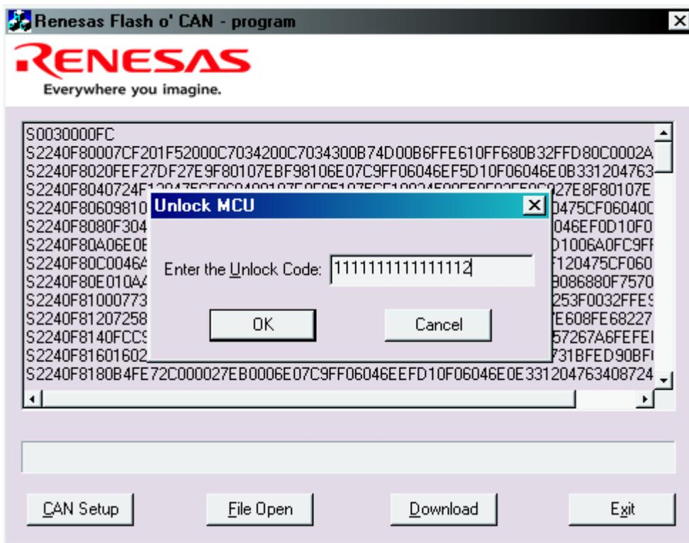
**Figure 3. The PC\_Download application. The Device Unlock Code is entered, after pressing ‘Download’. This example shows using the default Device Unlock Code for the RSK29.**
