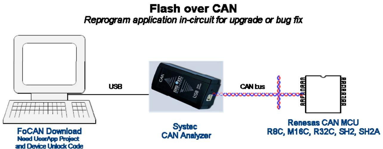
**Figure 1. Flash over CAN may be used to reflash an application after a device is installed by giving the device a unique programming ID.**
