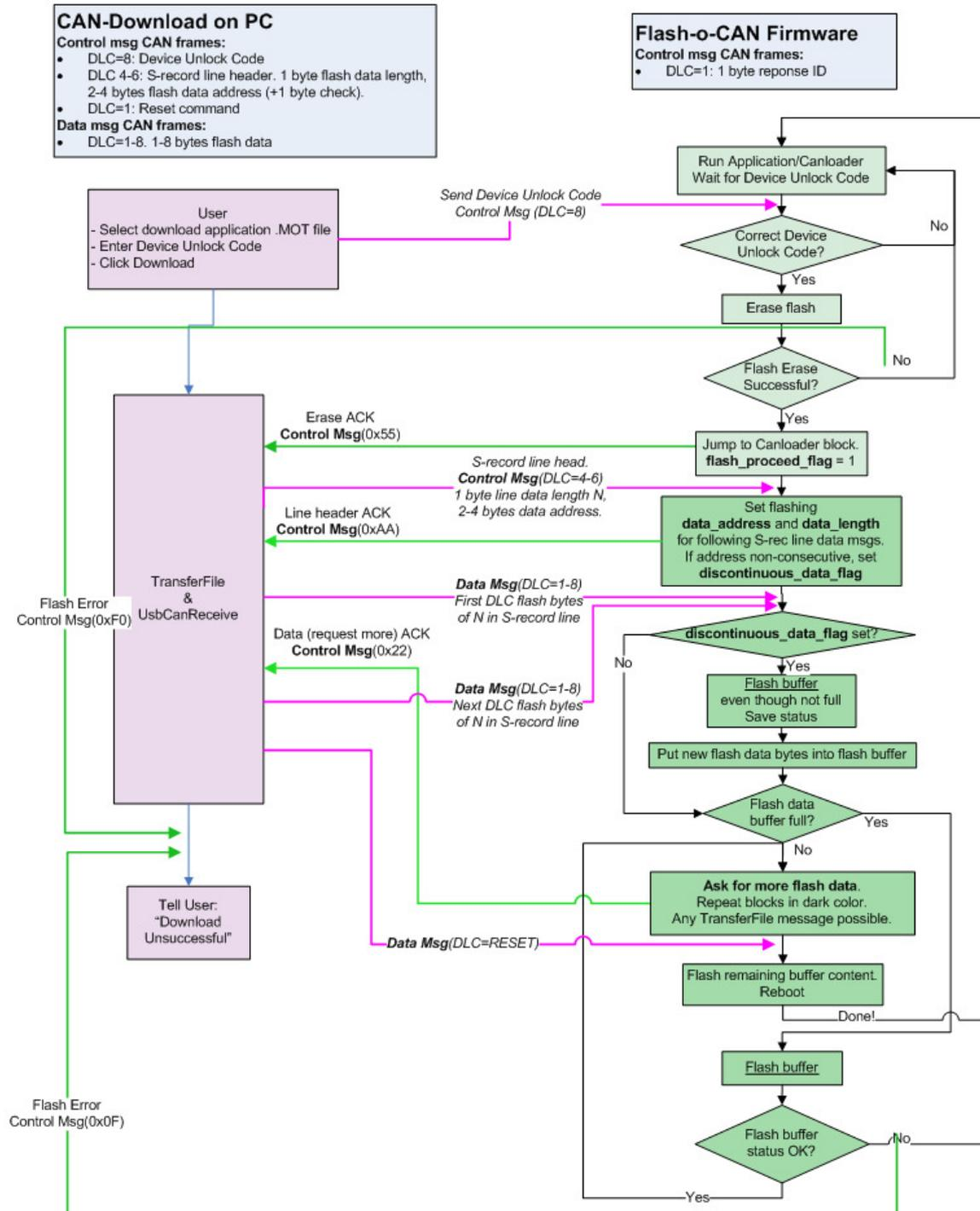
Figure 10. The Flash-over-CAN firmware download interaction process (protocol).
