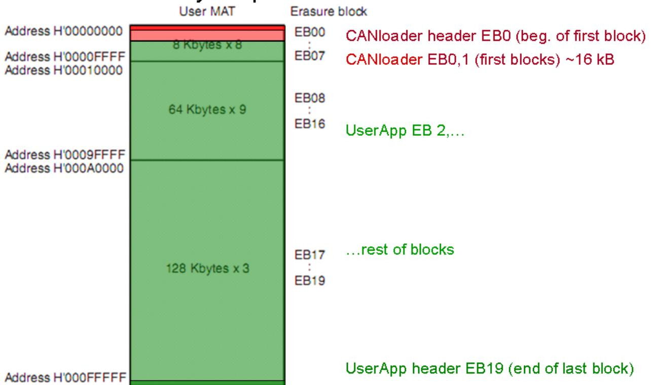
Figure 4 Flash o' CAN memory layout for an SH216 MCU.
