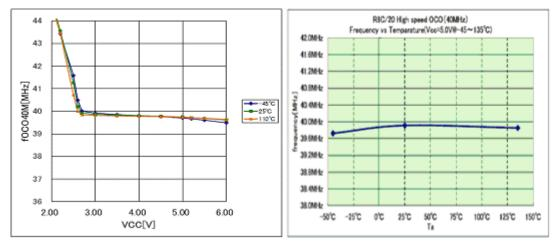
Figure 1: Effects of Operating Voltage and Temperature on HSOCO Frequency
