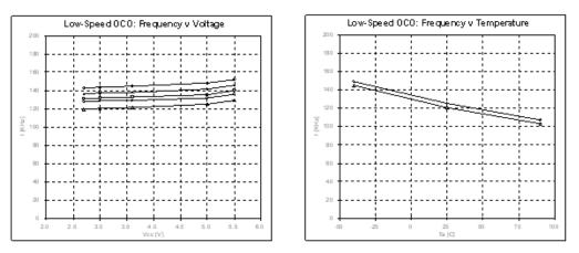
Figure 2: Effects of Operating Voltage and Temperature on HSOCO Frequency
