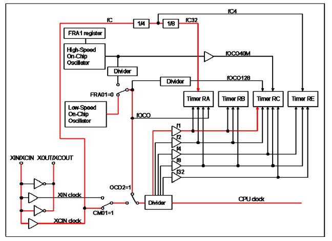
*Figure 4: Clock Generation Circuit, simplified to show Timer clock source options. Measuring the LSOCO using a 32 kHz XCIN as a reference.*
