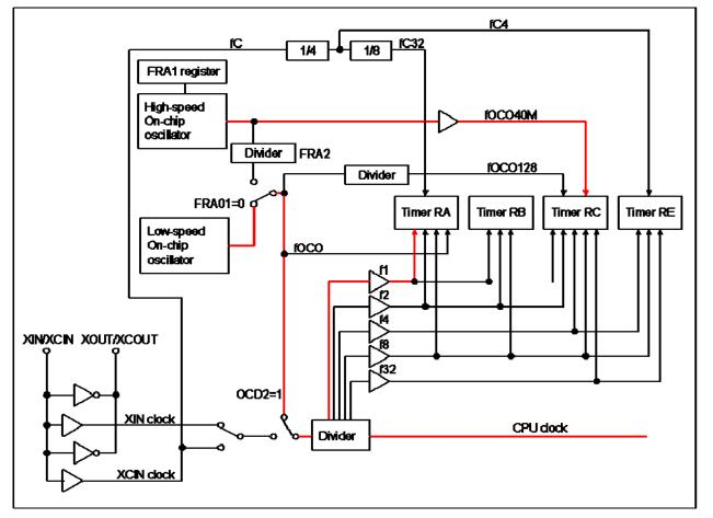
Figure 4: Clock Generation Circuit, simplified to show Timer clock source options. Measuring the LSOCO using the High-Speed On-Chip Oscillator as a reference.
