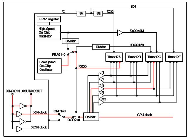
*Figure 3: Clock Generation Circuit, simplified to show Timer clock source options. Measuring the LSOCO using an external clock oscillator as a reference.*
