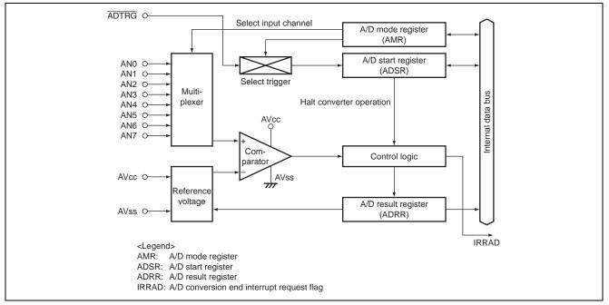
Figure 2 Block Diagram of A/D Converter
