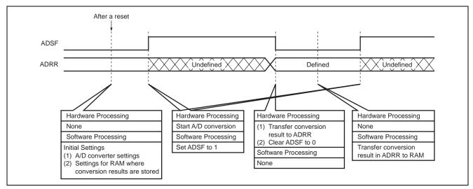
Figure 3 Principles of Operation of Voltage Measurement by A/D Conversion
