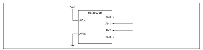
Figure 1 Voltage Measurement by 4-Channel A/D Conversion
