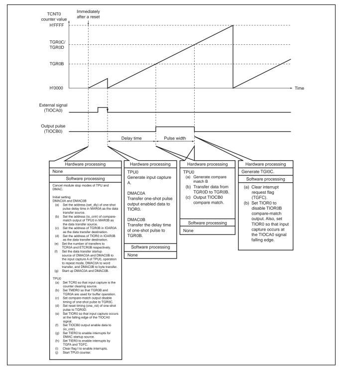
Figure 3 Principles of Operations Used of One-Shot Pulse Output
