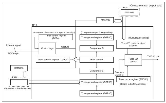
Figure 2 Block Diagram of One-Shot Pulse Output
