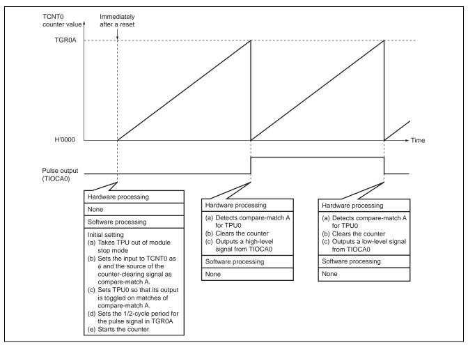
Figure 3 Principle of Pulse-Output Operation
