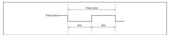
Figure 1 Example of Pulse Output
