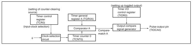
Figure 2 Configuration for Pulse-Train Output
