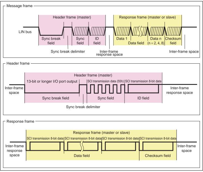
Figure 3 Message Frame Structure
