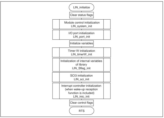
Figure 15 Initialization Function Flowchart
