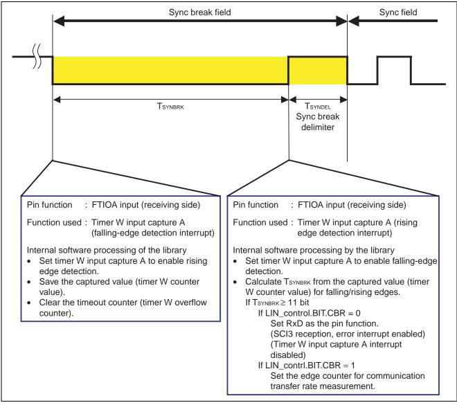
Figure 7 Detection of a Sync Break Field
