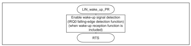
Figure 19 Flowchart of the Wake-up Signal Reception Preparation Function
