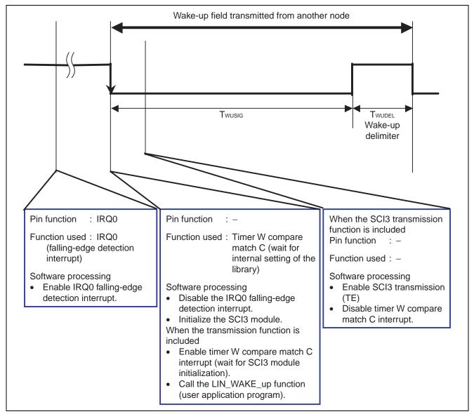
Figure 14 Reception of a Wake-up Signal
