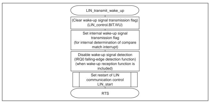
Figure 18 Flowchart of the Wake-up Signal Transmission Function
