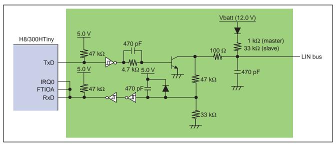
Figure 2 Sample LIN Bus Interface Circuit
