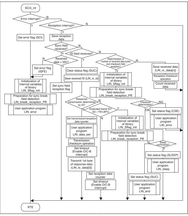
Figure 23 Flowchart of the SCI3 Interrupt Function
