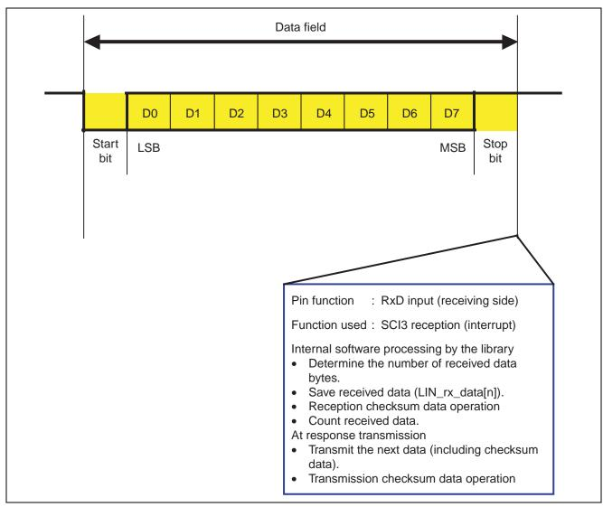
Figure 11 Transmission/Reception of a Data Field and Transmission of Checksum Data
