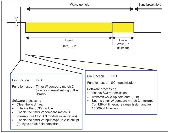
Figure 13 Transmission of a Wake-up Signal
