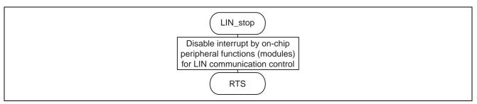
Figure 16 Flowchart of the LIN Communication Control Stop Function
