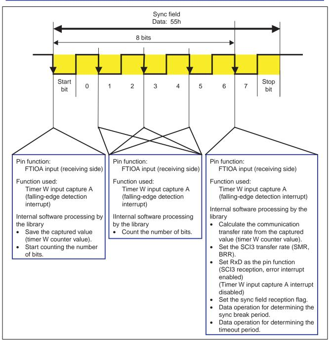
Figure 9 Correction of the Communication Transfer Rate by the Timer W Input Capture Function
