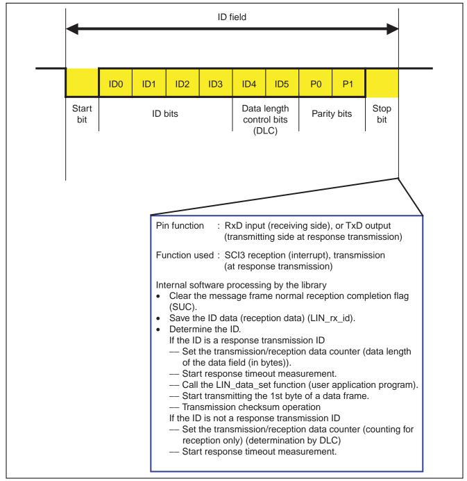
Figure 10 ID Field Reception and Determination
