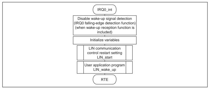
Figure 21 Flowchart of the IRQ Interrupt Function
