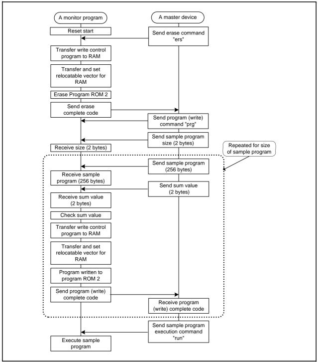
Figure 4.2 Monitor Program Operation Example
