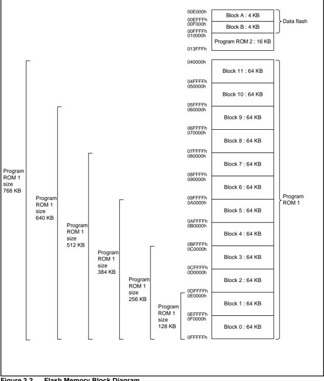
Figure 3.2 **Flash Memory Block Diagram**
