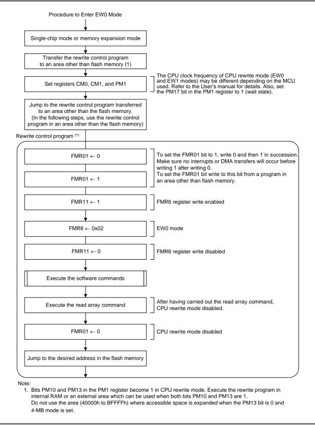
Figure 3.1 Settings and Resetting of EW0 Mode
