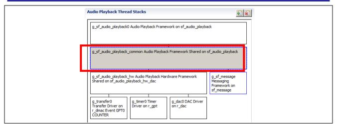
Change the property Audio Message Queue Name to the name of the queue identified previously: audio\_playback\_thread0\_message\_queue. This allows Audio Playback Framework module to be an Audio Playback Event Class subscriber.
