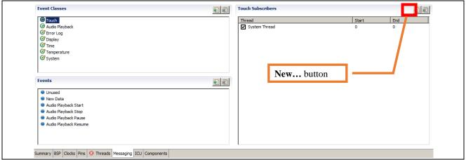
2. Shown below are examples of registered subscribers for each Event Classes. For instance, the Touch Event Class message is subscribed by the System Thread only in this example. The Audio Playback Event Class is subscribed by two threads, System Thread and Audio Playback Thread. (See section 4.4 for details about Audio Playback.)
