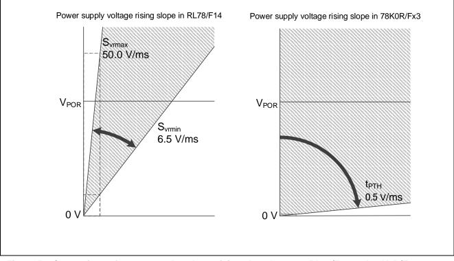
Figure 5-3 Comparison of power supply voltage rising slope between RL78/F14 and 78K0R/Fx3
