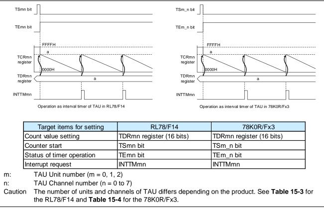
Figure 15-2 Comparison of operation as interval timer of TAU between RL78/F14 and 78K0R/Fx3
