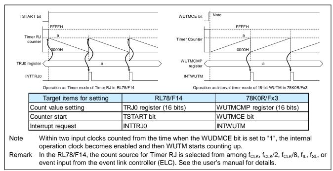
Figure 15-12 Comparison of 16-bit WUTM operation and Timer RJ operation
