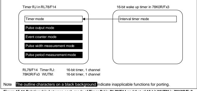
Figure 15-11 Relationship between each mode of Timer RJ in RL78/F14 and that of 16-bit WUTM in 78K0R/Fx3
