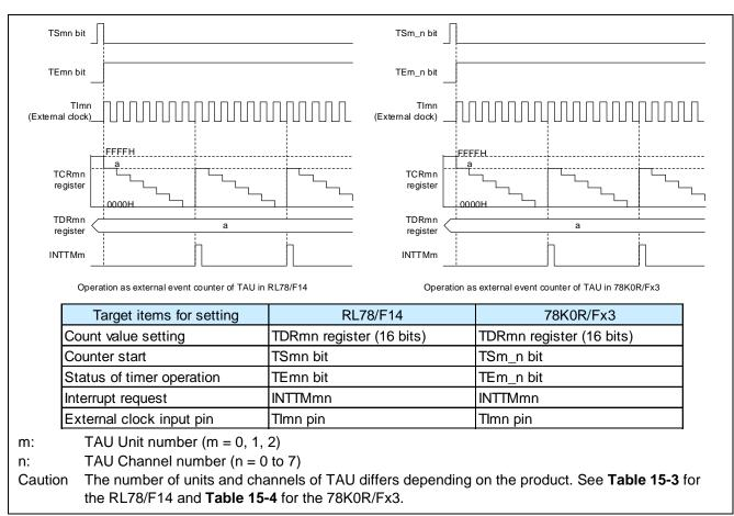
Figure 15-4 Comparison of operation as external event counter of TAU between RL78/F14 and 78K0R/Fx3
