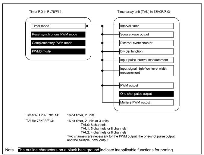
Figure 15-13 Relationship between each mode of Timer RD in RL78/F14 and that of TAU in 78K0R/Fx3
