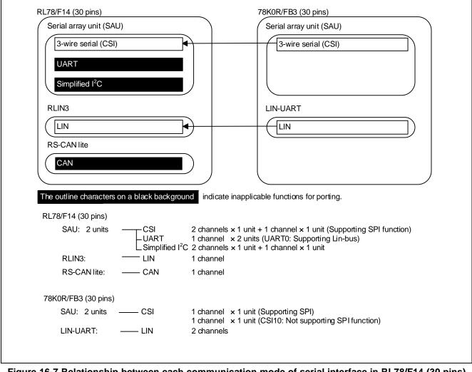
Figure 16-7 Relationship between each communication mode of serial interface in RL78/F14 (30 pins) and that in 78K0R/FB3 (30 pins)
