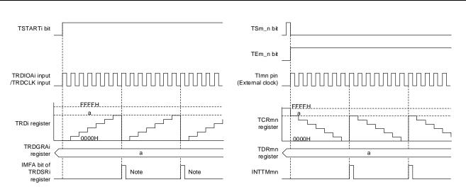
Example of operation as timer mode (Input capture function) of Timer RD in RL78/F14
