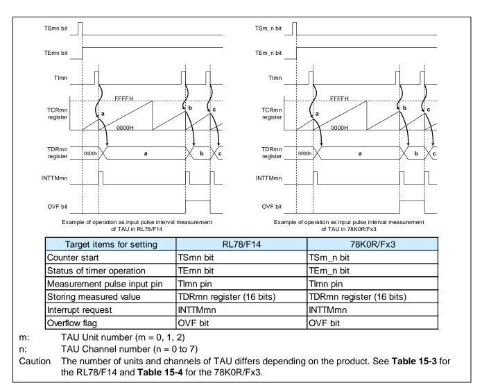
Figure 15-6 Comparison of operation as input pulse interval measurement of TAU between RL78/F14 and 78K0R/Fx3
