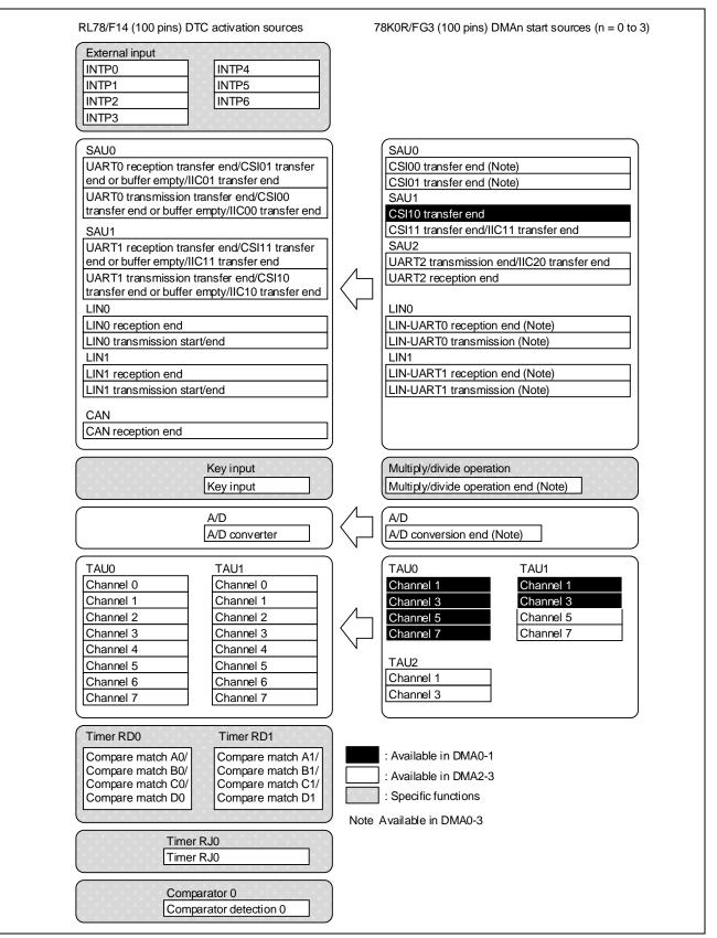
Figure 14-2 Comparison of functions between DTC activation sources in RL78/F14 (100 pins) and DMA start sources in 78K0R/FG3
