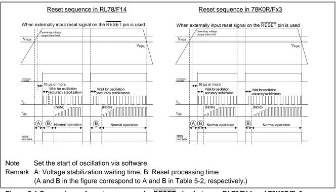
Figure 5-1 Comparison of reset sequences by RESET pins between RL78/F14 and 78K0R/Fx3
