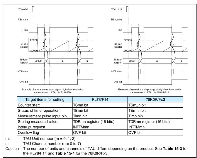
Figure 15-7 Comparison of operation as input signal high-/low-level width measurement of TAU between RL78/F14 and 78K0R/Fx3
