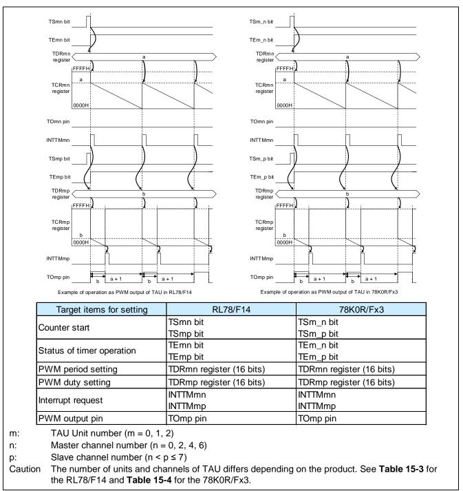
Figure 15-9 Comparison of operation as PWM output between RL78/F14 and 78K0R/Fx3
