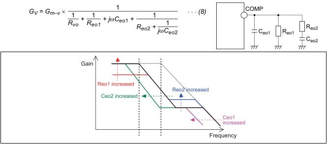
Figure 12 Overview of Gain–Frequency Characteristics
