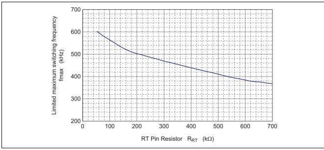
Figure 9 RT Pin Resistor vs. Limited Maximum Switching Frequency
