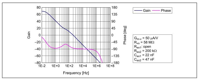
Figure 13 Frequency Characteristics of the Error Amplifier
