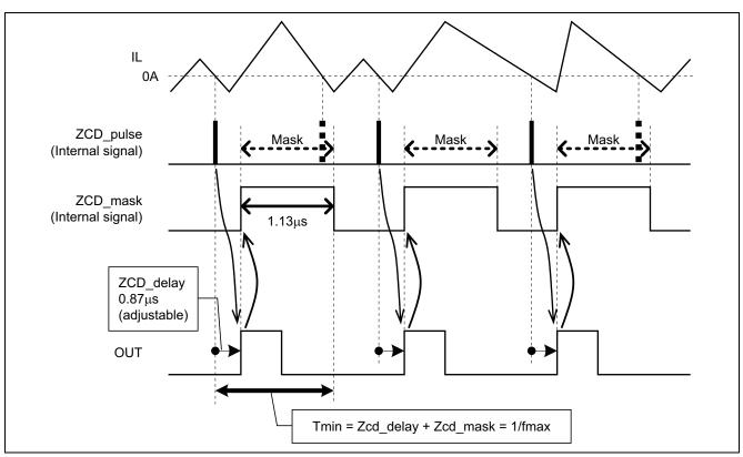
Figure 8 Waveform at Limited Maximum Switching Frequency Operation
