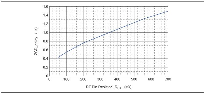
Figure 2 RT Pin Resistor vs. ZCD\_dealy Time
