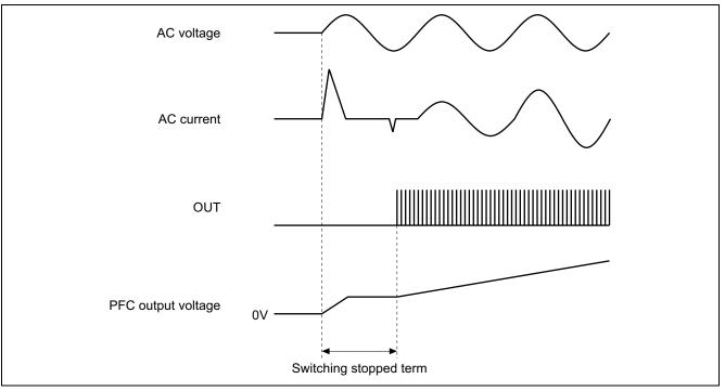
Figure 10 Example(1) Stop of the Switching Operation
