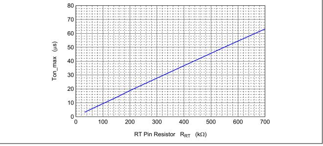
Figure 11 RT Pin Resistor (R<sub>RT</sub>) vs. Ton\_max
