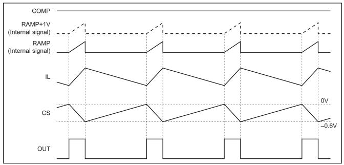
Figure 7 Waveform at the Over Current Detection
