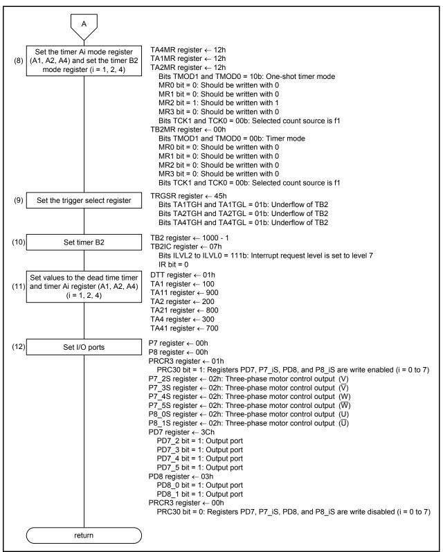
Figure 6.7 Initial Setting of the Three-Phase Motor Control Timers (2/2)
