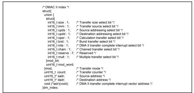
Figure 6.2 Structure/Union Used in the Sample Code
