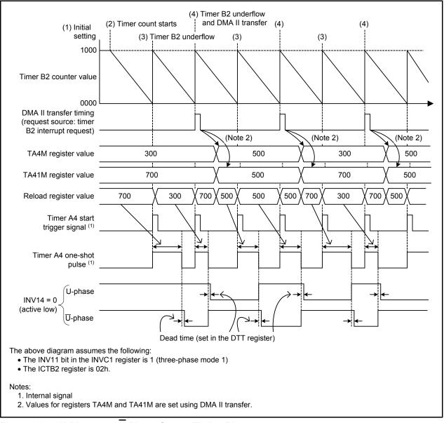
Figure 6.1 U-Phase and U-Phase Output Timing Diagram
