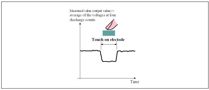
Figure 1-6 An example of measured value output
