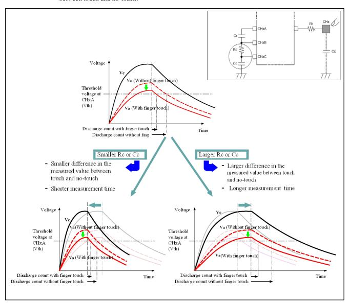
Figure 2-1 Variation of measured values due to changed Rc or Cc
