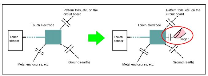
Figure 1-1 Increased floating capacitance due to the presence of a finger
