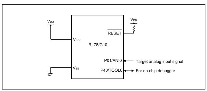
Figure 4.1 Hardware Configuration
