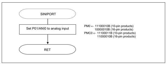
Figure 5.3 I/O Port Setup Function
