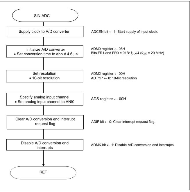
Figure 5.5 A/D Converter Setup
