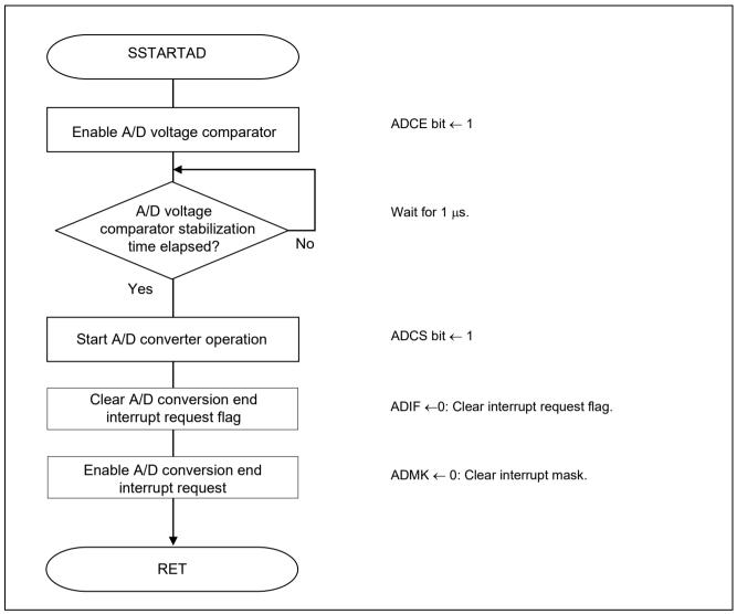
Figure 5.7 A/D Conversion Start Processing
