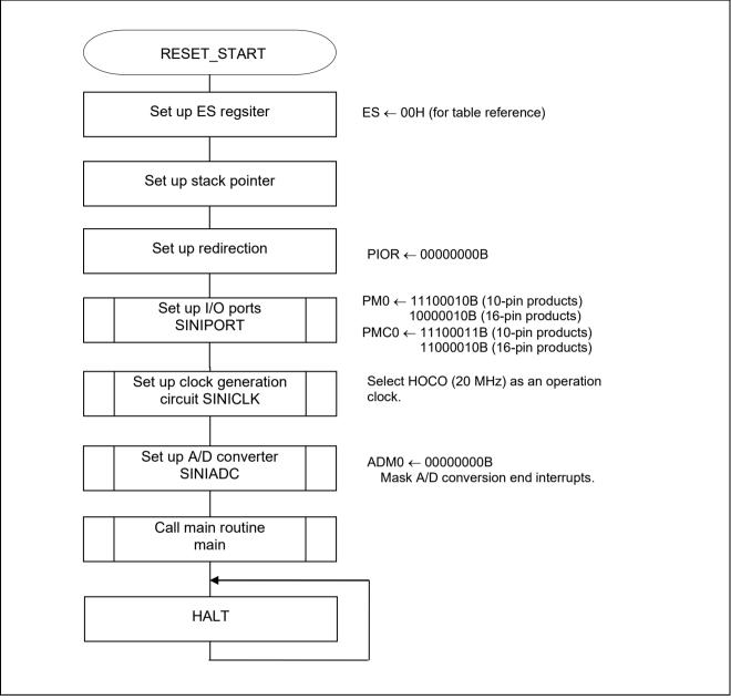
Figure 5.2 CPU Initialization Function
