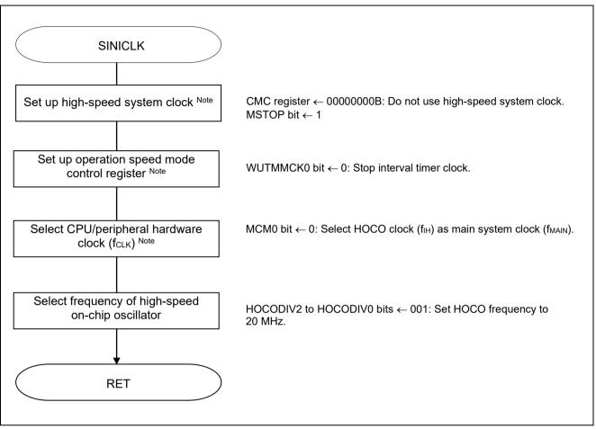
Figure 5.4 Clock Generation Circuit Setup
