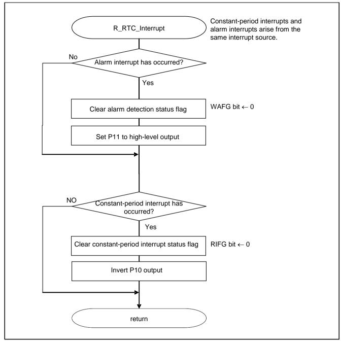
Figure 5.14 RTC Interrupt (INTRTC) Processing
