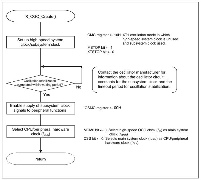
Figure 5.5 CPU Clock Setup
