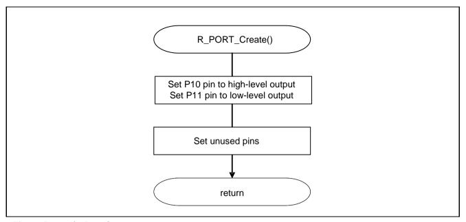
Figure 5.4 I/O Port Setup
