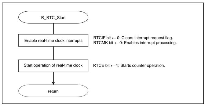
Figure 5.10 RTC Startup
