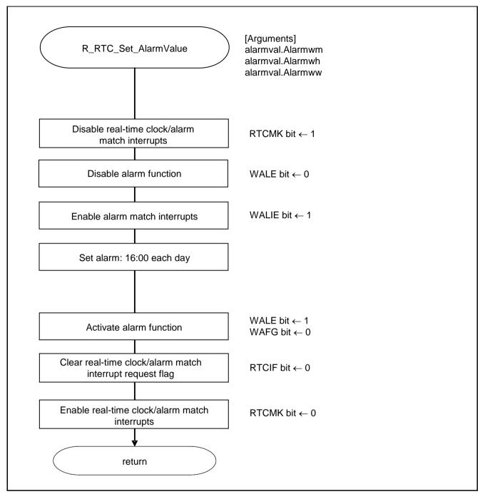
Figure 5.13 Alarm Generation Time Setup
