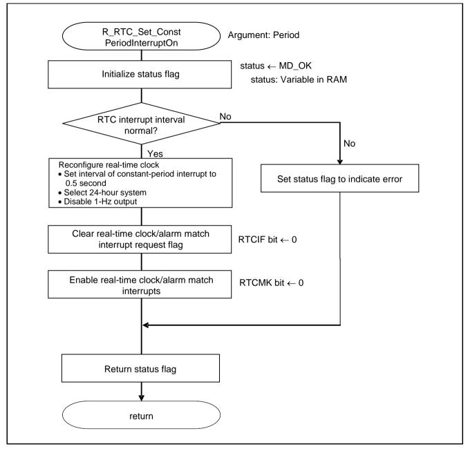
Figure 5.9 RTC Reconfiguration
