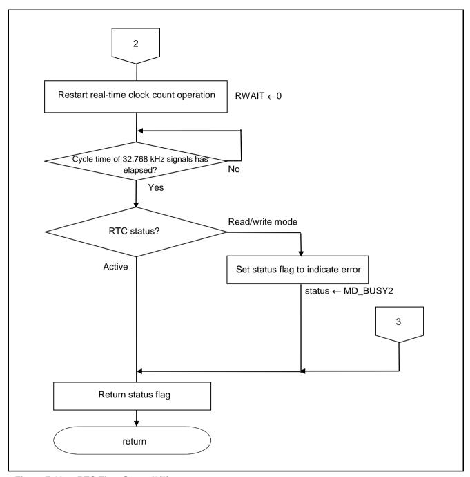
Figure 5.12 RTC Time Setup (2/2)
