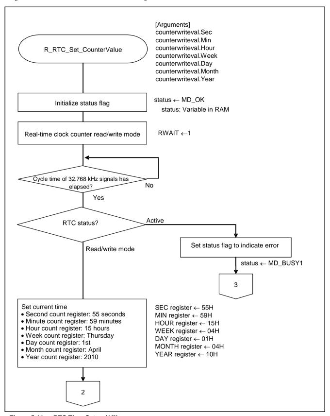
Figure 5.11 RTC Time Setup (1/2)
