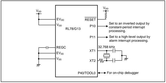
Figure 4.1 Hardware Configuration
