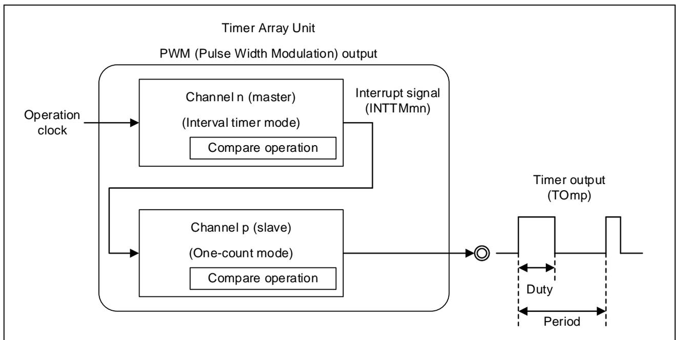
**Figure 5.1 Operation Overview (example of migration from timer mode (output compare function) or PWM mode)**
