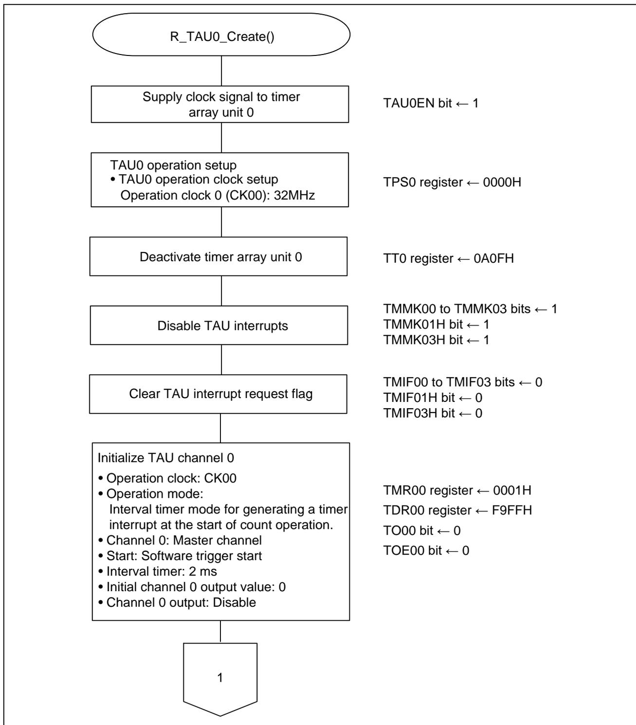
Figure 5.9 Timer Array Unit Setup (1/2)
