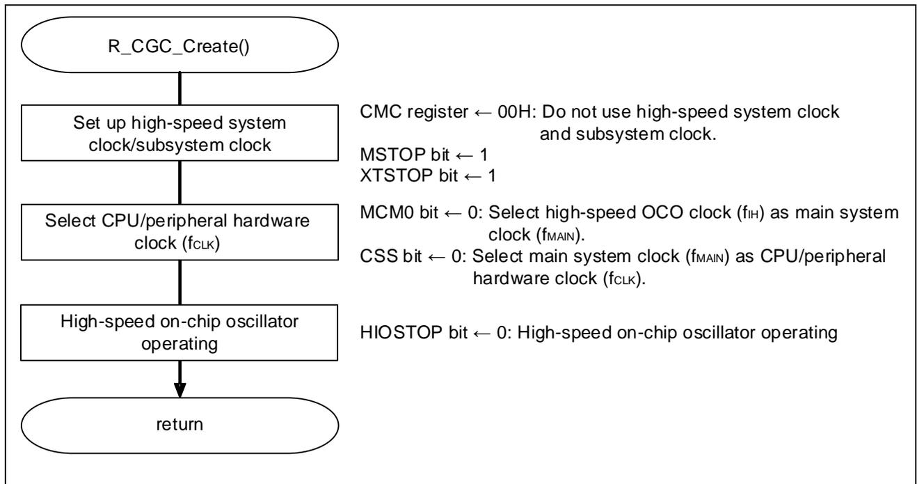
Figure 5.7 CPU Clock Setup
