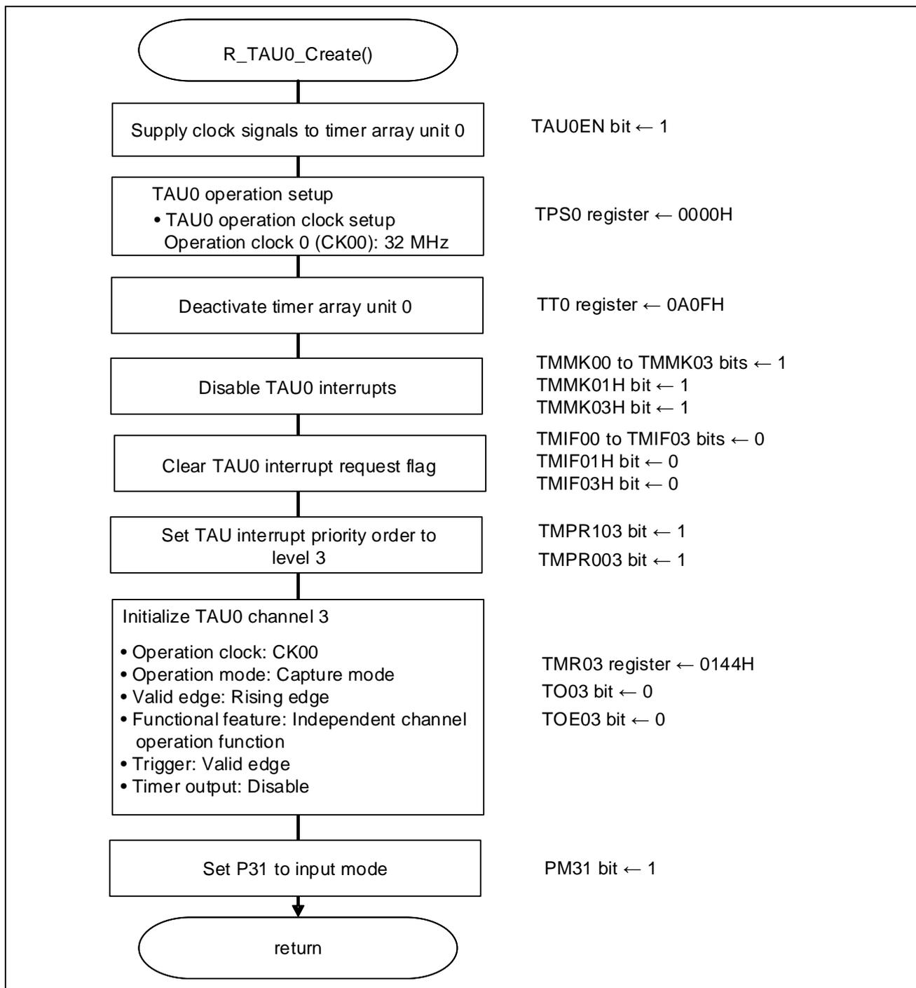
Figure 4.9 Timer Array Unit Setup
