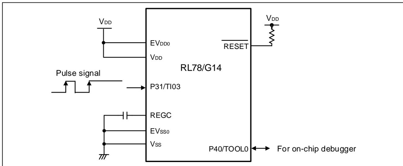
**Figure 4.2 Hardware Configuration**
