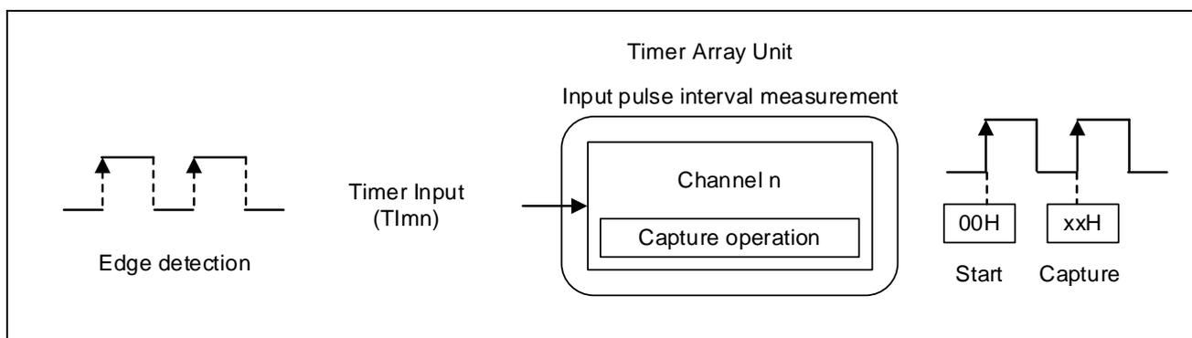
**Figure 4.1 Operation Overview (Example of Migration from Timer Mode (Input Capture Function))**
