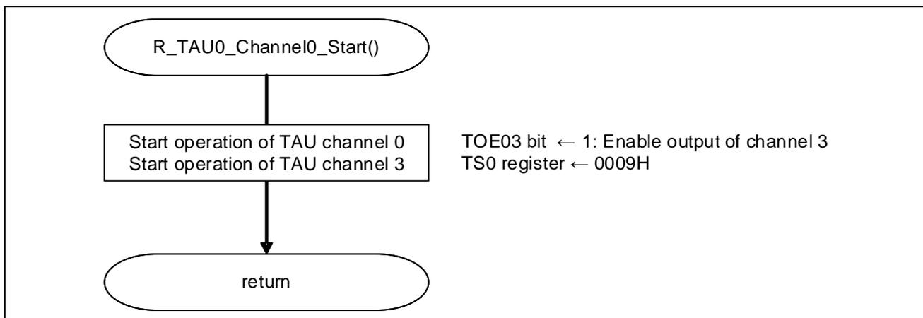
Figure 5.12 Timer Array Unit Operation Start
