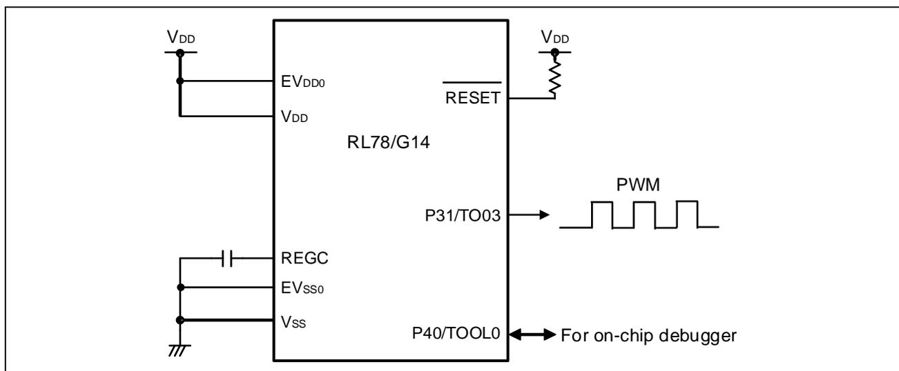
**Figure 5.2 Hardware Configuration**
