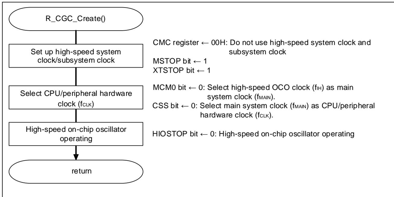
Figure 4.7 CPU Clock Setup
