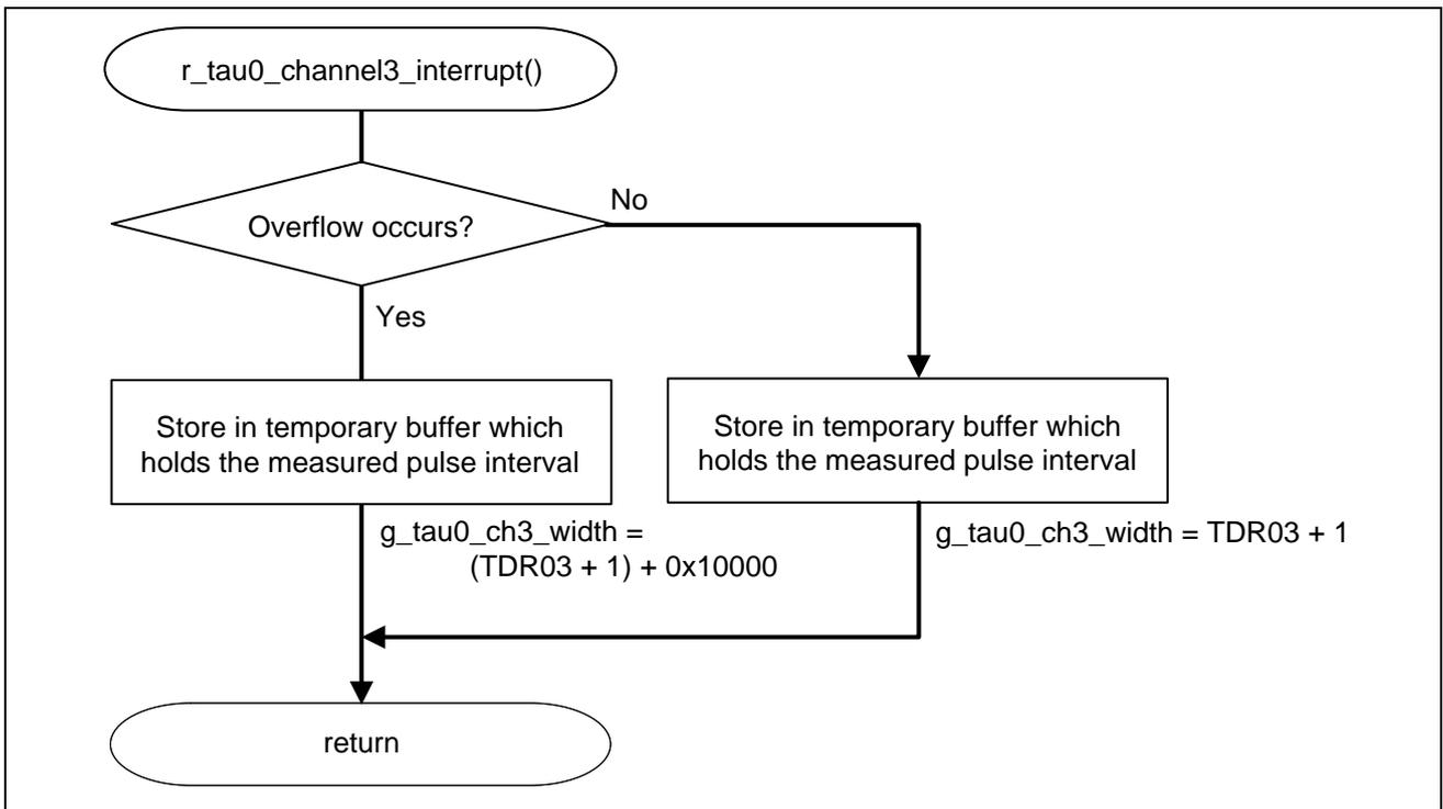
Figure 4.12 INTTM03 Interrupt Processing
