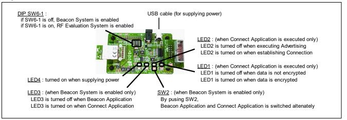
Figure 4-2 Evaluation Board Operation
