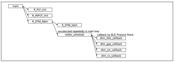
Figure 7-2 Function Calling Graph of RF Evaluation Operation
