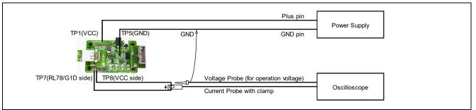
Figure 4-3 Measurement Environment which uses Current Probe
