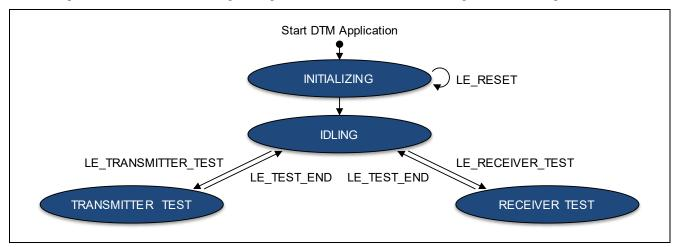
Figure 8-3 State Transition of DTM Application
