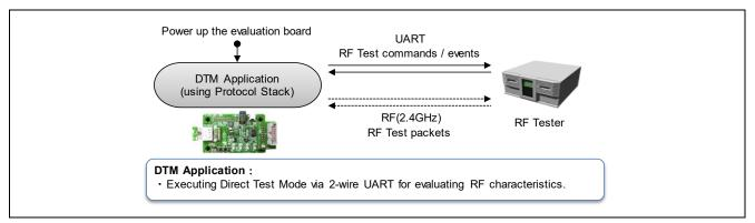
Figure 1-3 Overview of RF Evaluation Operation
