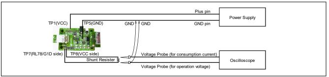
Figure 4-4 Measurement Environment which uses the combination of Shunt Resistor and Voltage Probe
