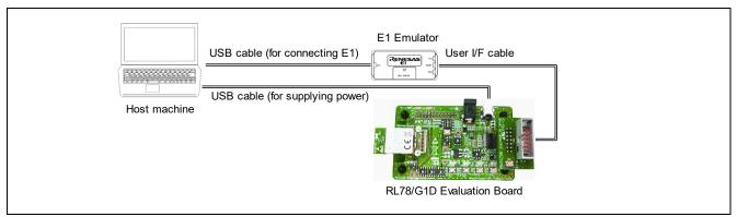
Figure 4-1 Evaluation Board Operation
