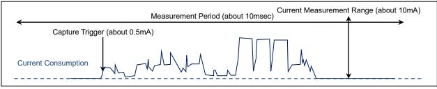
Figure 4-5 Measuring Current Consumption in Periodic Packet Transmission
