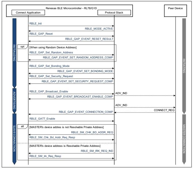
Figure 8-5 Initializing & Advertising & Slave Connection (Configurations) Sequence of Connect Application
