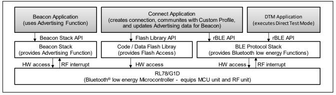
Figure 1-1 Architecture of Sample Program
