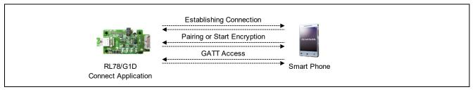
Pushing SW2 on the evaluation board can change Beacon Application and Connect Application alternately when the Sample Program is running in Beacon Operation. When Connect Application works, not only LED4 but also LED3 are turned on. Connect Application transmits connectable advertising packet in order to connect peer device. By connecting Smart Phone to RL78/G1D device and accessing GATT, it is possible to update Advertising data Beacon Application transmits.
