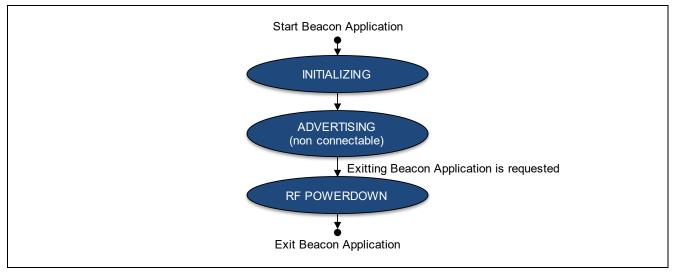
Figure 8-1 State Transition of Beacon Application
