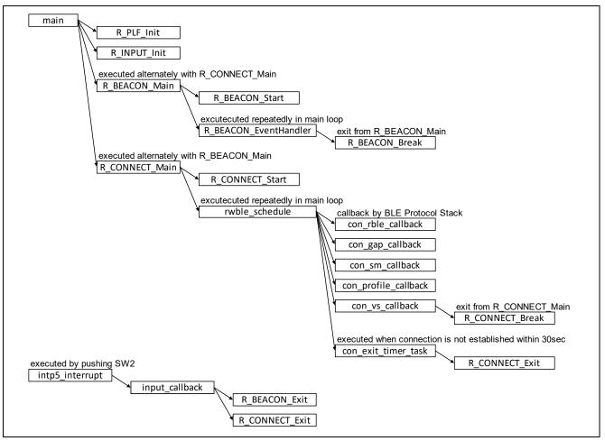
Figure 7-1 Function Calling Graph of Beacon Operation
