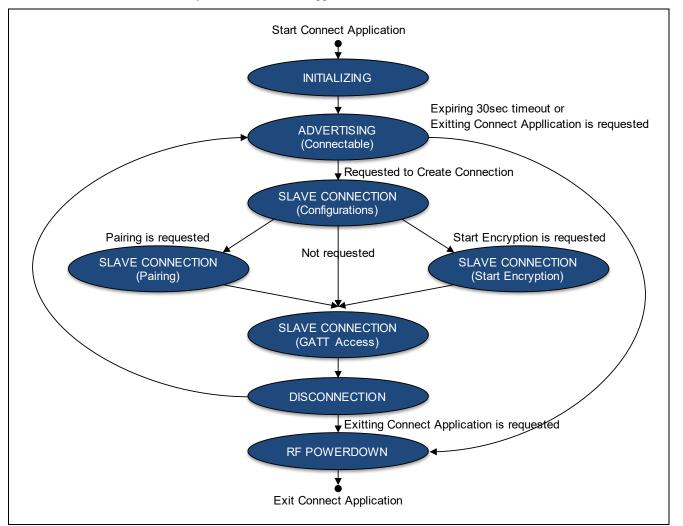
Figure 8-2 State Transition of Connect Application
