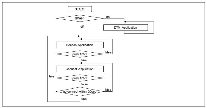
Figure 6-1 Application Switch Operation when the Sample Program uses switches on the evaluation board
