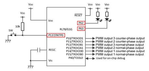
G1G Target Board Hardware Configuration
