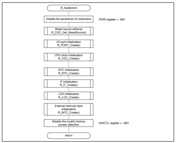
Figure 5.5 Peripheral Function Initialization
