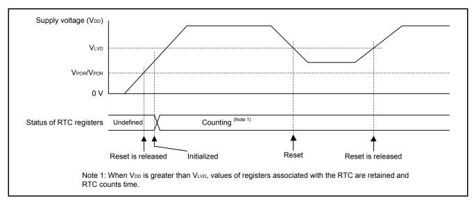
Figure 1.1 Operation Overview of Supply Voltage Shift and Data Retention
