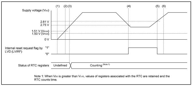
Figure 5.2 Operation Overview of Supply Voltage Shift and RTC Status
