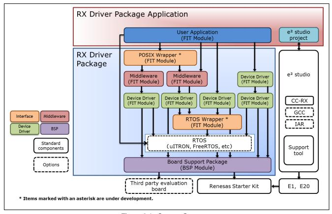
Figure 2-1 System Structure
