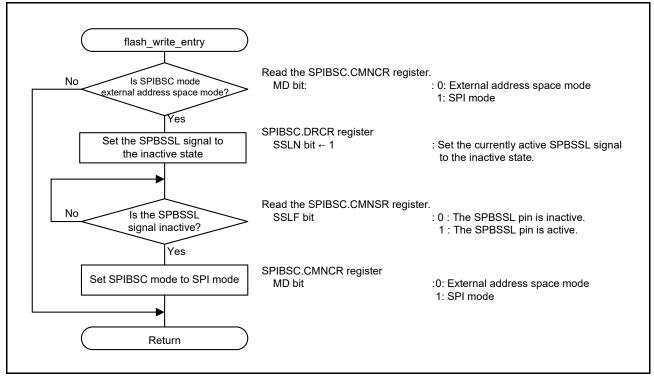
Figure 7.2 Flow of the Serial Flash Memory Write Mode Entry Function
