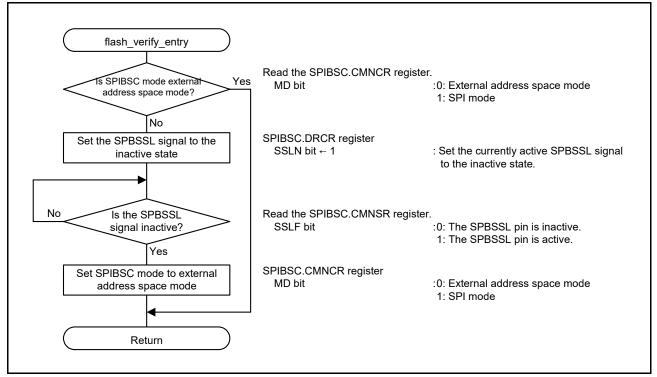
Figure 7.3 Flow of the Serial Flash Memory Read Mode Entry Function
