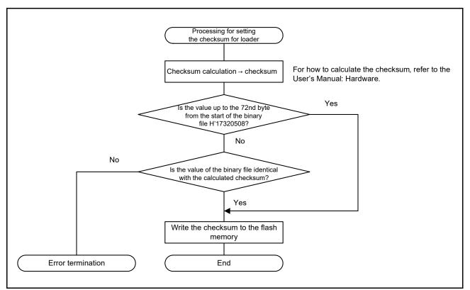
Figure 8.5 Flow of Processing for Setting the Checksum of the Loader Parameter Information
