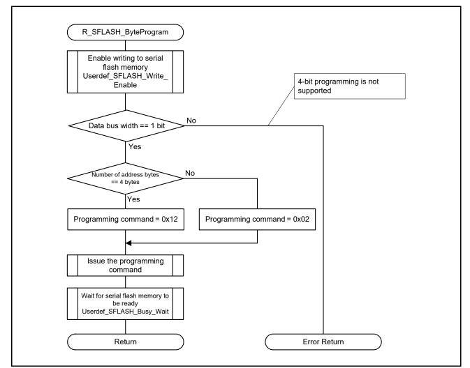
Figure 10.14 Flow of Programming the Serial Flash Memory
