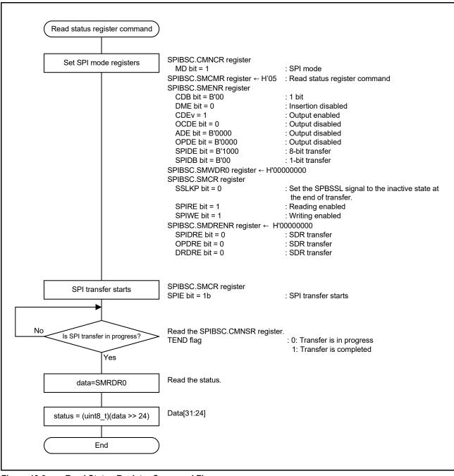
Figure 10.6 Read Status Register Command Flow
