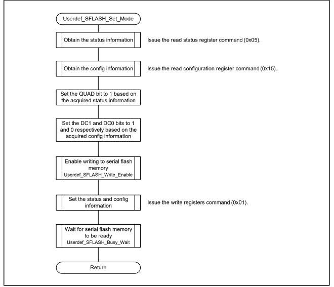
Figure 10.5 Flow of Setting the Registers in the Serial Flash Memory
