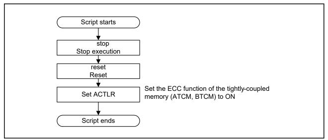
Figure 9.1 Details of Processing by the RZ/T1 Evaluation Board Initialization Script
