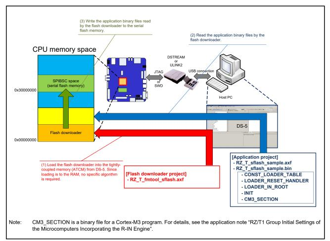
Figure 5.1 Schematic View of Flash Downloader Operation
