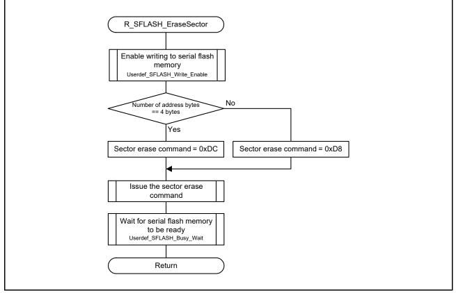
Figure 10.12 Flow of Erasing the Serial Flash Memory
