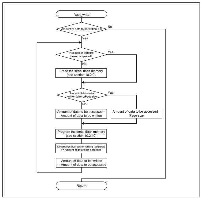
Figure 7.4 Flow of the Serial Flash Memory Write Function
