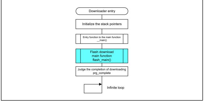
Figure 8.2 Flash Downloader Processing Flow (1/3)
