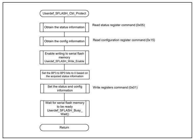
Figure 10.11 Flow of Releasing the Serial Flash Memory from Protection
