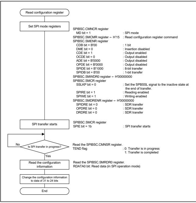
Figure 10.7 Read Configuration Register Command Flow
