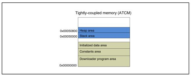
Figure 5.3 Memory Allocation of the Flash Downloader
