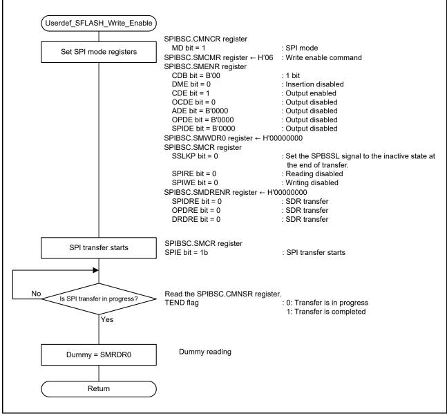
Figure 10.9 Flow of Enabling Writing to the Serial Flash Memory
