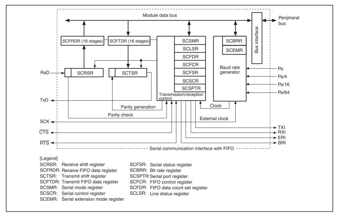
Figure 1 SCIF Block Diagram
