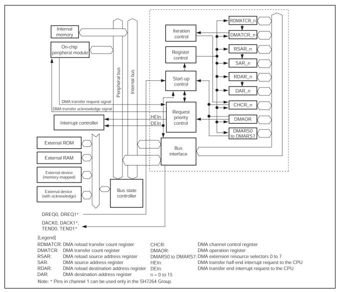
Figure 2 DMAC Block Diagram
