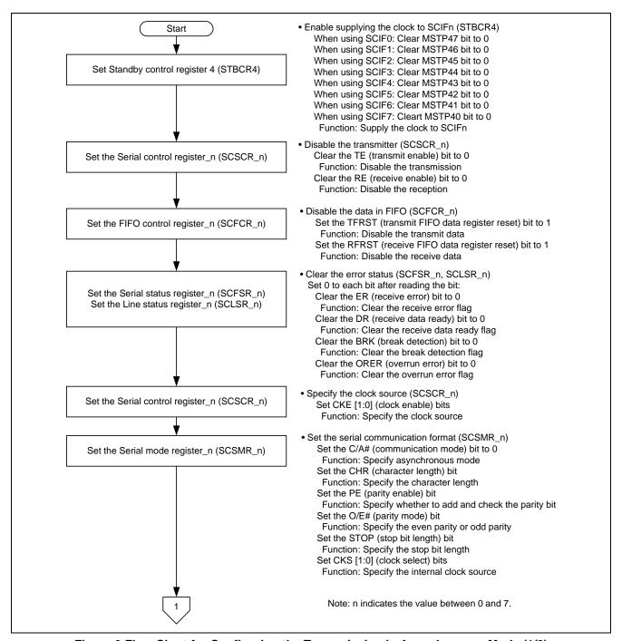
Figure 3 Flow Chart for Configuring the Transmission in Asynchronous Mode (1/2)
