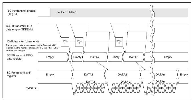
Figure 6 Transmission Timing in the Sample Program
