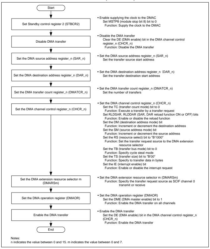
Figure 5 Flow Chart for Configuring the DMAC
