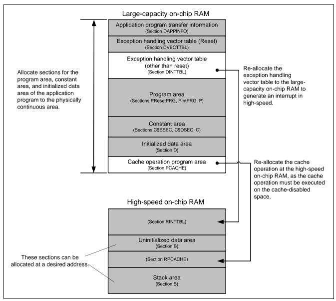
**Figure 8 Application Program Section Alignment**
