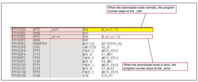
Figure 18 High-performance Embedded Workshop Window When the Downloader Ends
