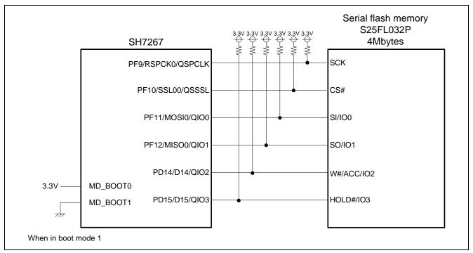
**Figure 4 Serial Flash Memory Circuit**
