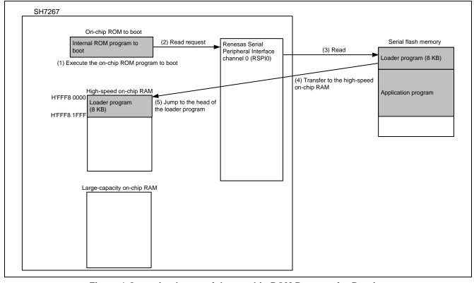
Figure 1 Operation Image of the on-chip ROM Program for Booting
