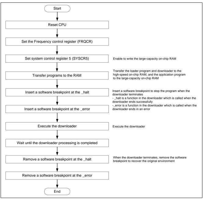
Figure 15 Command Batch File Flow Chart
