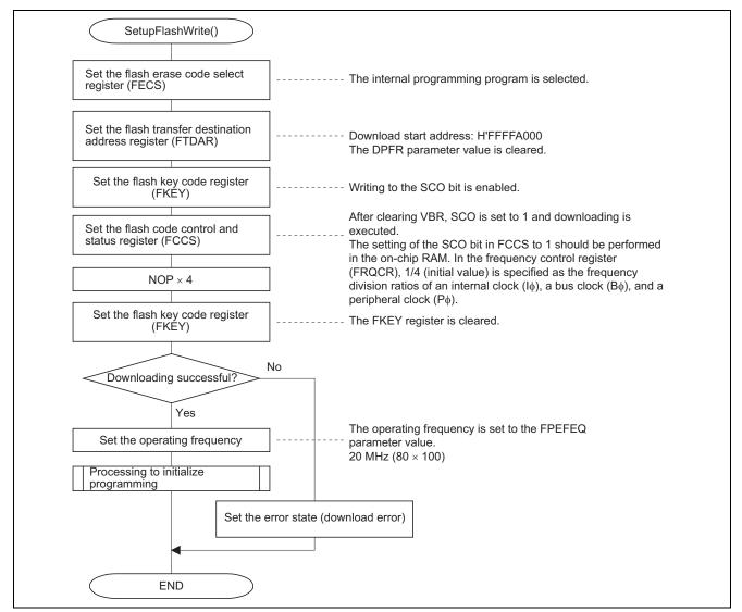
Figure 16 Processing by the Programming Program Downloading and Initialization Routine
