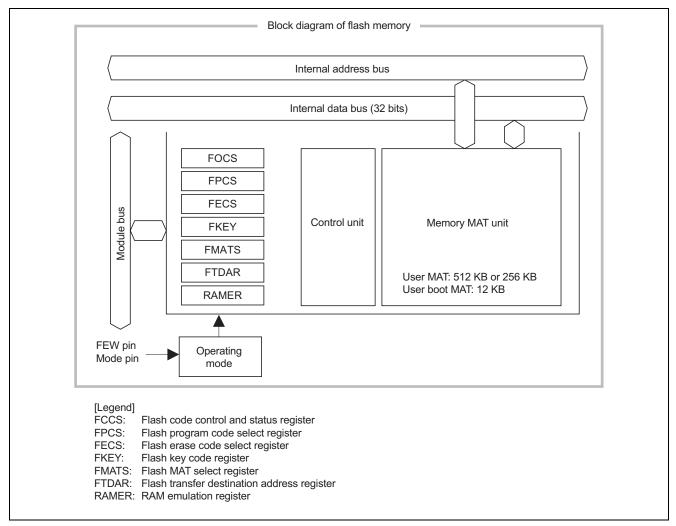
Figure 2 Block Diagram of Flash Memory
