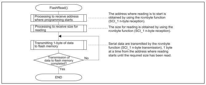
Figure 13 Processing to Read Flash Memory
