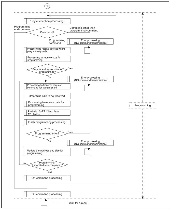
Figure 12 Processing by the Main Routine for Flash Programming (2)
