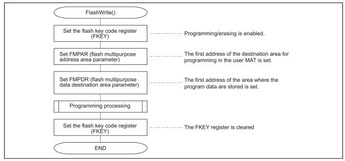
Figure 17 Processing by the Flash Programming Routine Processing
