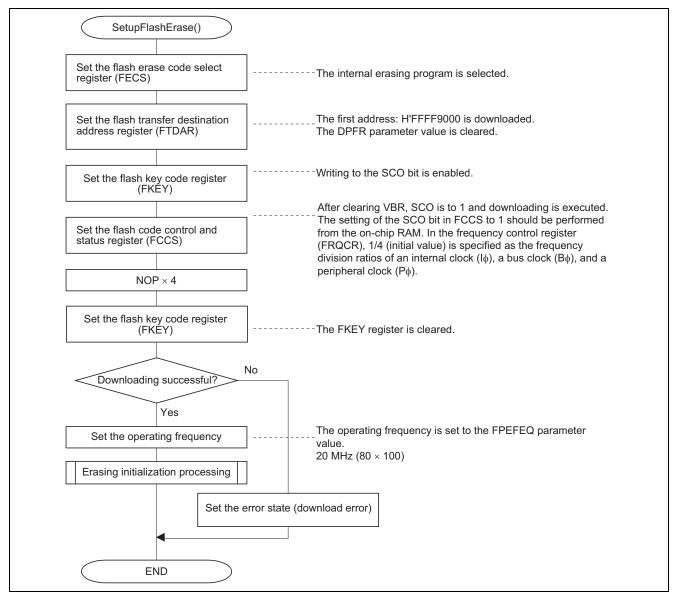
Figure 14 Processing by the Erasing Program Downloading and Initialization Routine
