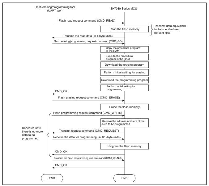
Figure 5 Control Sequence for Commands
