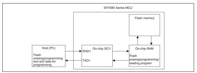
Figure 1 Erasing and Programming Flash Memory in User Program Mode
