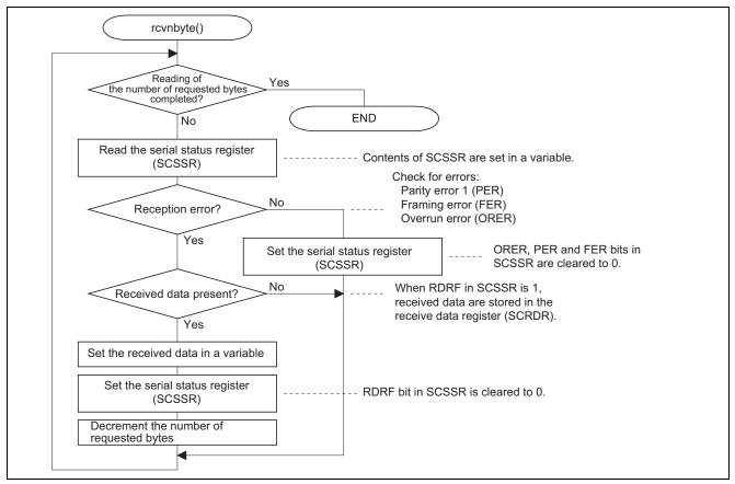
Figure 9 Processing by the SCI\_1 n-Byte Reception Routine
