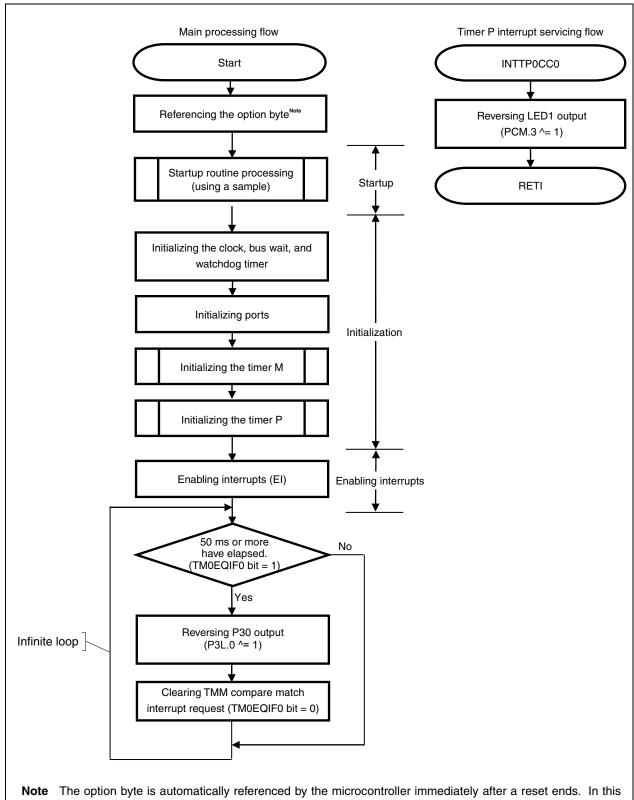
**Note** The option byte is automatically referenced by the microcontroller immediately after a reset ends. In this sample program, the oscillation stabilization time immediately after a reset ends is set to 6.554 ms using the option byte.
