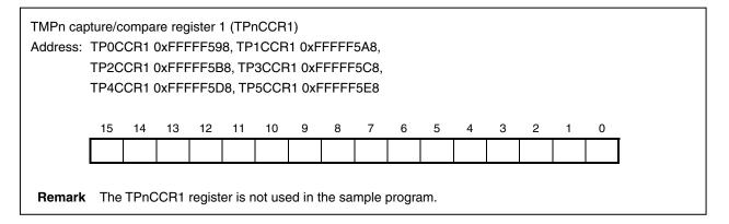
Four capture/compare registers (TQ0CCR0 to TQ0CCR3) are provided for 16-bit timer/event counter Q (TMQ). These registers are used in the same way as the TPnCCR0 and TPnCCR1 registers.
