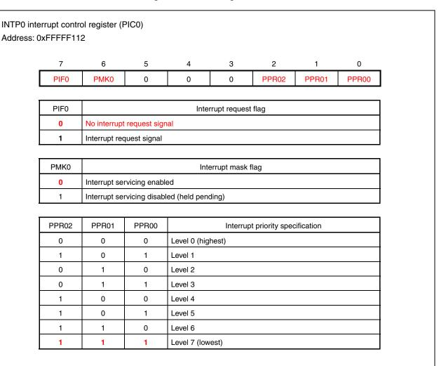
Figure 4-13. PIC0 Register Format
