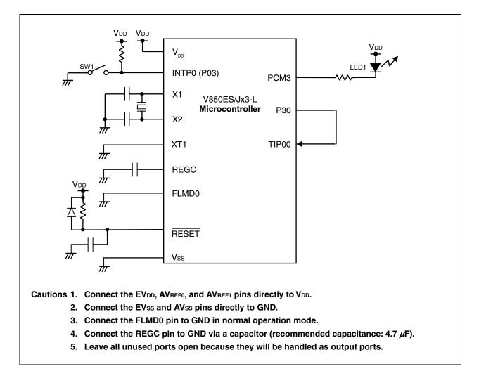
Figure 2-1. Circuit Diagram
