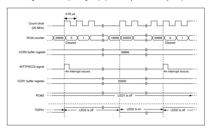
Figure 4-10. PWM Output Timing Example (When PWM Cycle Is 2 ms and Duty Is 50%)
