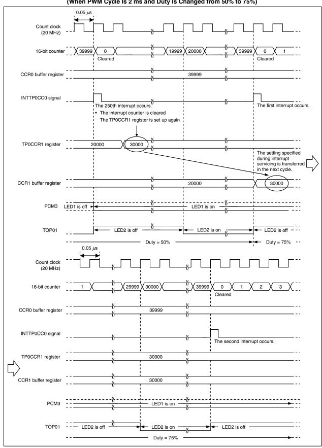
Figure 4-11. PWM Output Timing Example (When PWM Cycle Is 2 ms and Duty Is Changed from 50% to 75%)
