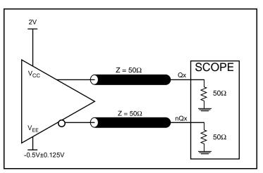
2.5V LVPECL Output Load AC Test Circuit
