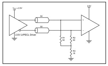
Figure 6B. 2.5V LVPECL Driver Termination Example
