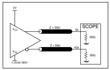
3.3V LVPECL Output Load AC Test Circuit
