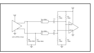
Figure 3E. PCLK/nPCLK Input Driven by a 2.5V LVPECL Driver with AC Couple
