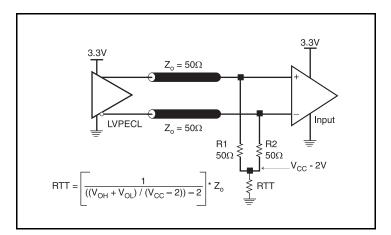
Figure 5A. 3.3V LVPECL Output Termination
