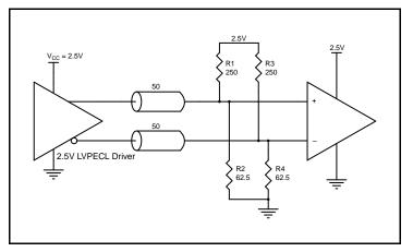
Figure 6A. 2.5V LVPECL Driver Termination Example
