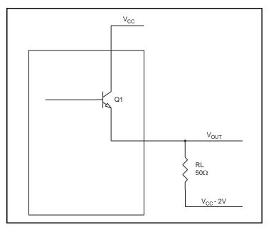
Figure 8. LVPECL Driver Circuit and Termination
