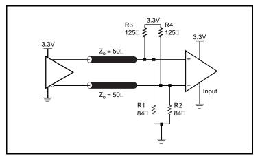
Figure 5B. 3.3V LVPECL Output Termination
