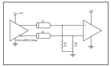
Figure 6C. 2.5V LVPECL Driver Termination Example
