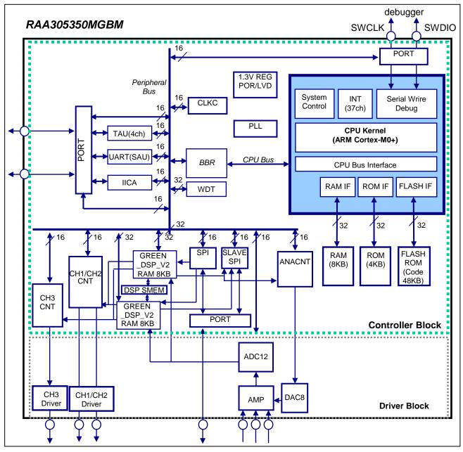
Figure 1.1 RAA305350MGBM Block diagram
