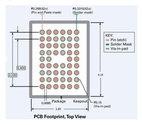
Figure 9. P9225-R Recommended PCB Footprint Dimensions in mm
