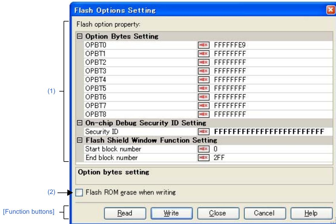
Figure A-57. Flash Options Setting Dialog Box [Simulator]
