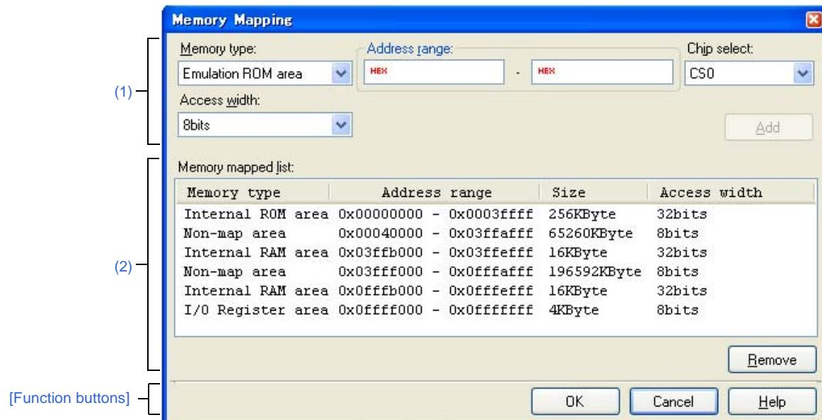
Figure A-52. Memory Mapping Dialog Box [Simulator]
