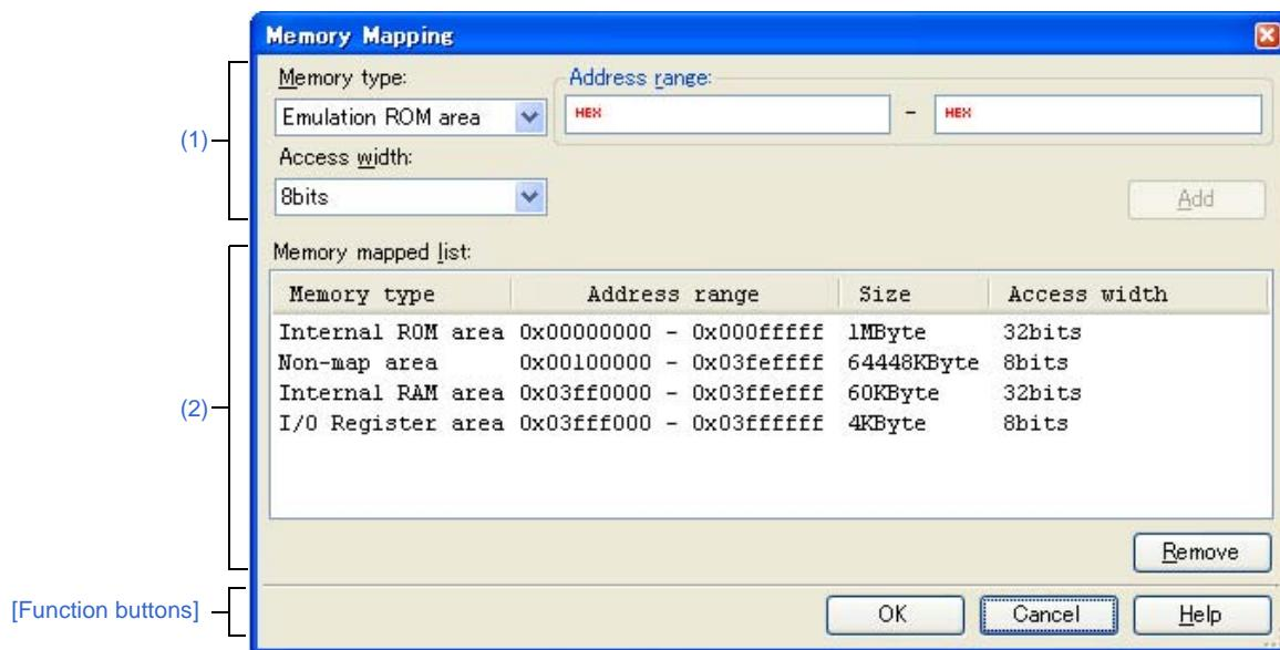
Figure A-51. Memory Mapping Dialog Box [IECUBE[V850E1]]
