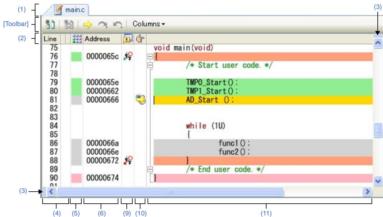
Figure A-28. Editor Panel (When Mixed Display Mode Is Selected)
