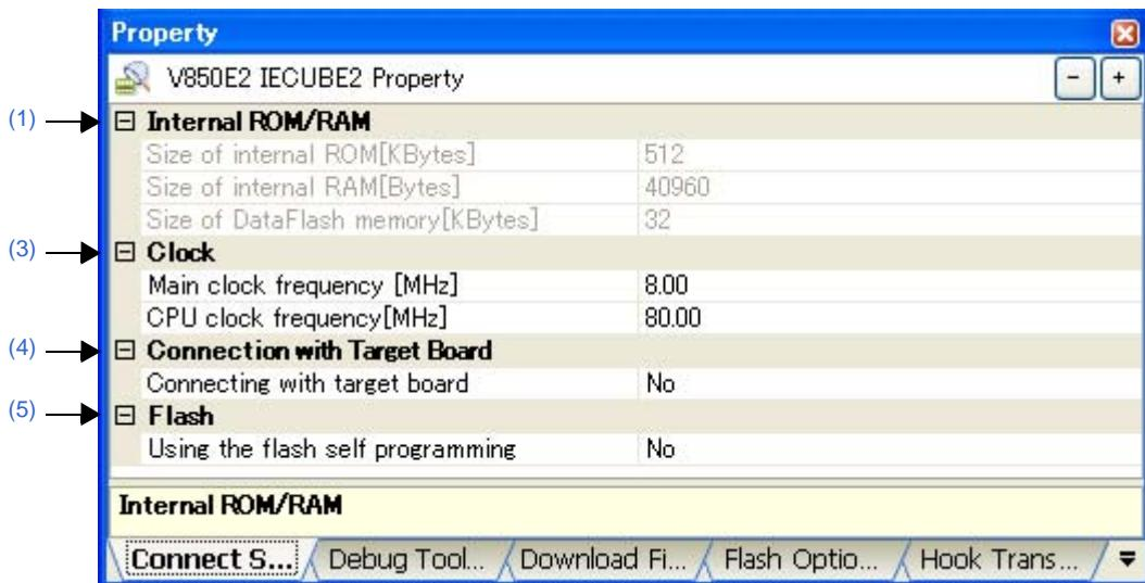
Figure A-8. Property Panel: [Connect Settings] Tab [MINICUBE][E1/E20(JTAG)] ([V850E1][V850ES])
