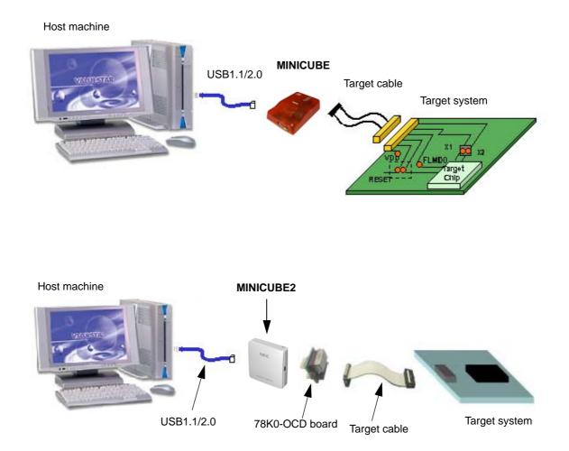
Figure 1-3 Example of ID78K0-QB System Configuration (MINICUBE)
