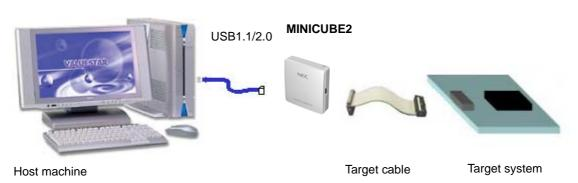
Figure 1-4 Example of ID850QB System Configuration [MINICUBE2]
