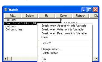
Figure 5-2 Setting Break to Variable
