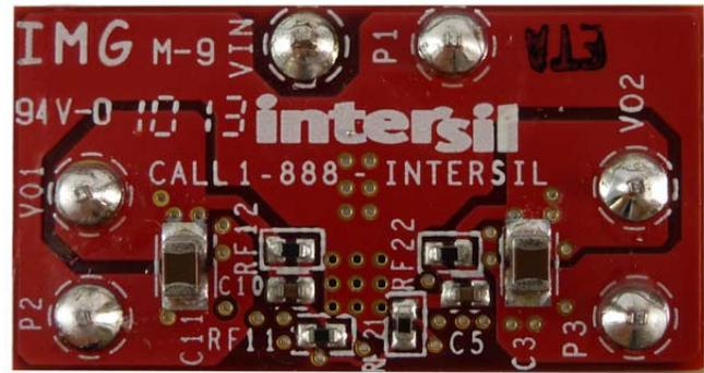
FIGURE 3. ISL8033DEMO1Z BOTTOM OF BOARD (Note 1)
