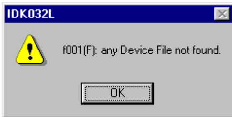
Figure 5-1 Error On No Device Files Installed
