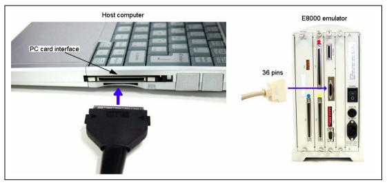
Figure 4 Connecting the PC Card Interface to the E8000 Emulator
