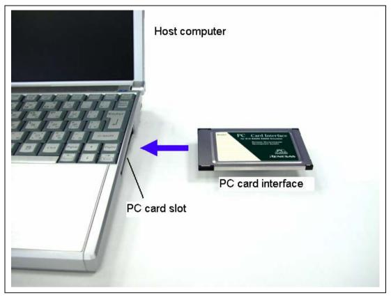
Figure 1 Connecting the PC Card Interface to the Host Computer
