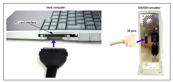
Figure 3 Connecting the PC Card Interface to the E6000H Emulator
