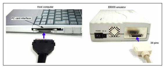
Figure 2 Connecting the PC Card Interface to the E6000 Emulator
