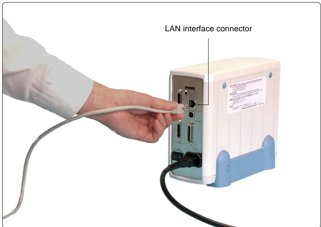
*Figure 4.4 Connecting LAN interface cable (emulator PC4701U side)*
