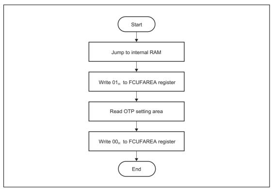
Figure 6.27 Flow of Reading the OTP Setting Area
