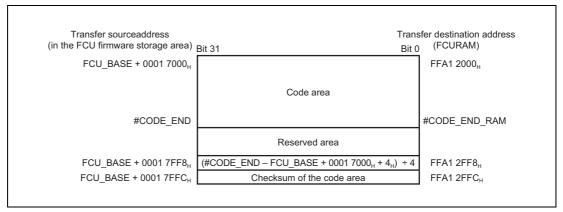
Figure 6.4 Configuration of FCU Firmware
