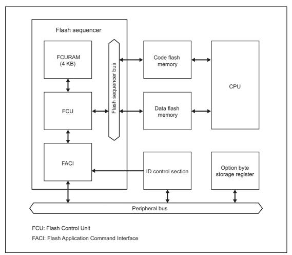
Figure 2.1 Configuration of Flash Memory Related Modules
