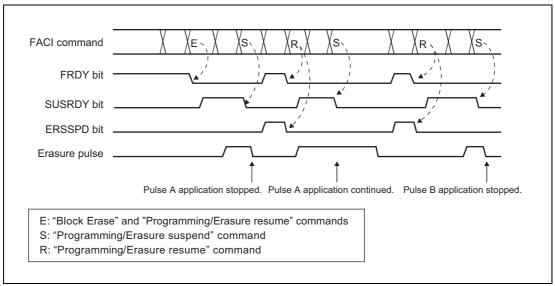
Figure 6.15 Suspend "Erase" Command (Suspension-Priority Mode)
