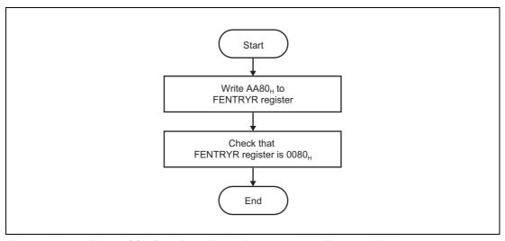
Figure 6.6 Flow of Shift to Data Flash Programming/Erasure Mode
