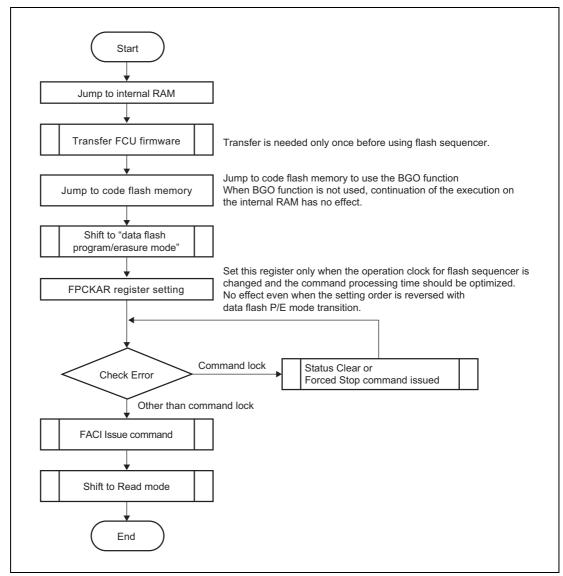
Figure 6.2 Overview of Command Usage in Data Flash Programming/Erasure Mode
