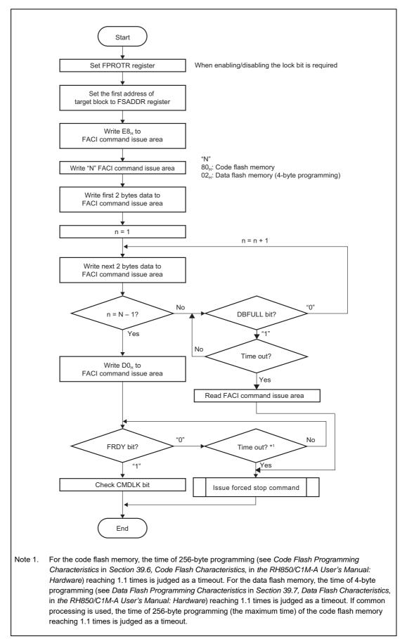
Figure 6.10 Programming Command Usage
