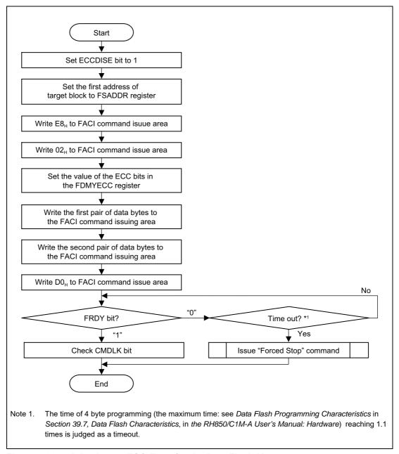
Figure 6.29 Injecting an ECC Error for the Data Flash Memory
