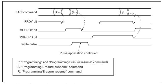
Figure 6.14 Suspend Programming Command
