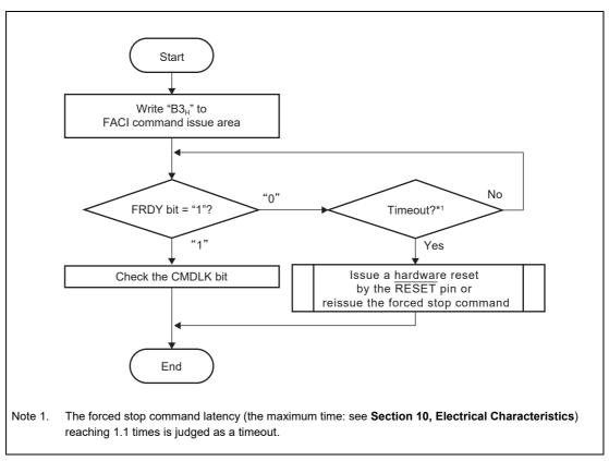
Figure 6.19 "Forced Stop" Command Usage
