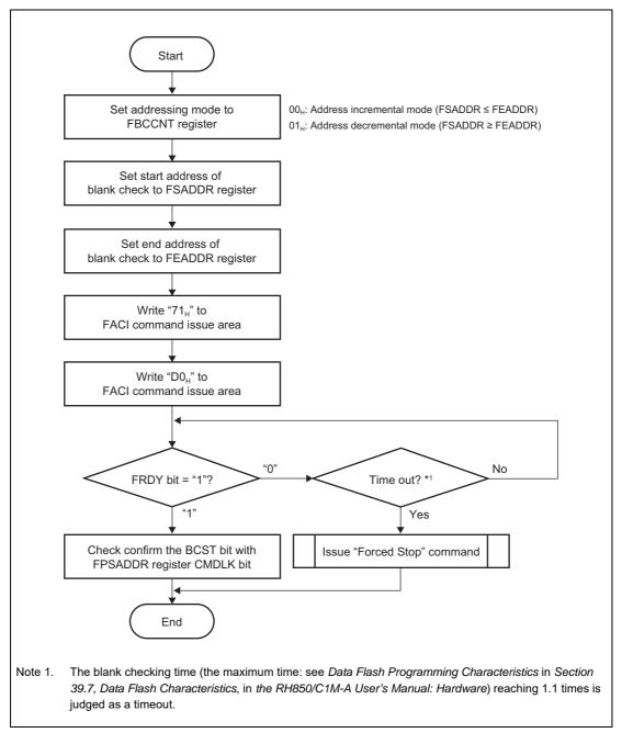
Figure 6.20 "Blank Check" Command Usage
