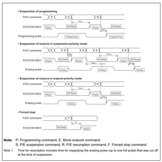
Figure 10.1 Timing of Suspension/Resumption/Forced Stop
