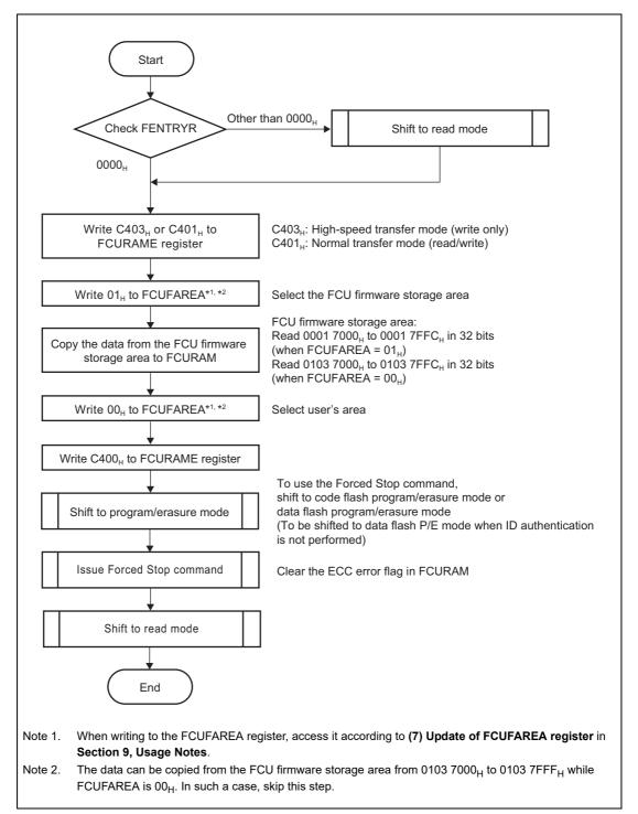
Figure 6.3 Transfer Flow of FCU Firmware
