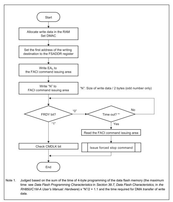
Figure 6.11 DMA Programming Command Usage
