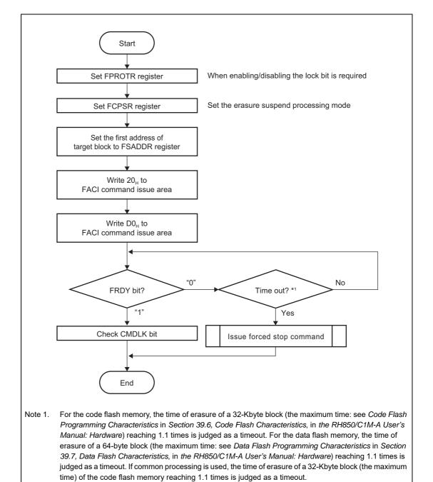
Figure 6.12 Block Erase Command Usage
