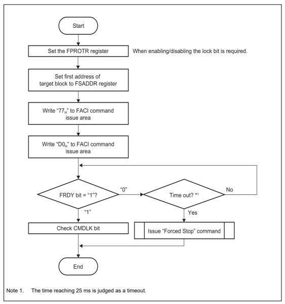
Figure 6.23 "Lock Bit Programming" Command Usage
