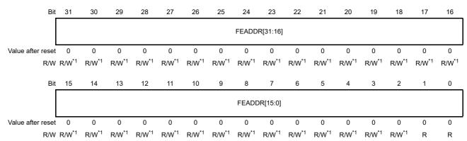
Note 1. This bit can be written when the FRDY bit in the FSTATR register is "1". Writing to this bit while the FRDY bits is "0" is ignored.
