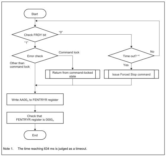
Figure 6.7 Flow of Shift to Read Mode
