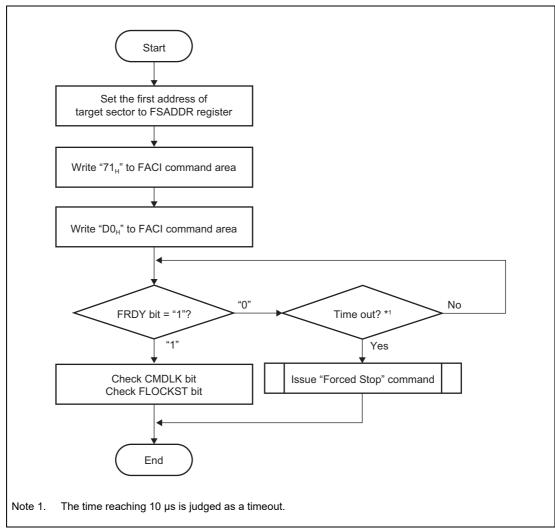
Figure 6.24 "Lock Bit Read" Command Usage
