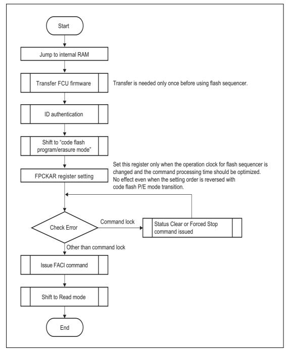
Figure 6.1 Overview of Command Usage in Code Flash Programming/Erasure Mode
