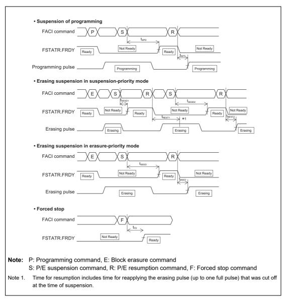
Figure 10.2 Timing of Suspension/Resumption/Forced Stop
