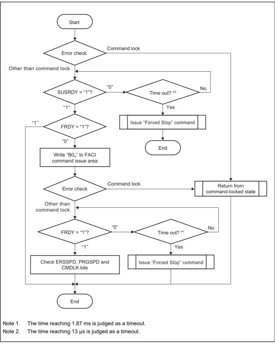
Figure 6.13 "Programming/Erasure Suspend" Command Usage
