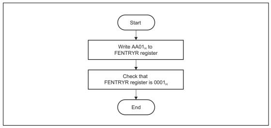
Figure 6.5 Flow of Shift to Code Flash Programming/Erasure Mode
