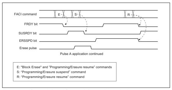
Figure 6.16 Suspend "Erase" Command (Erasure-Priority Mode)
