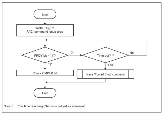
Figure 6.17 "Programming/Erasure Resume" Command Usage
