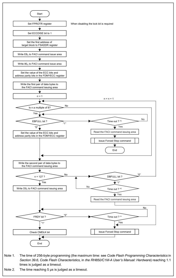
Figure 6.28 Injecting an ECC Error for the Code Flash Memory
