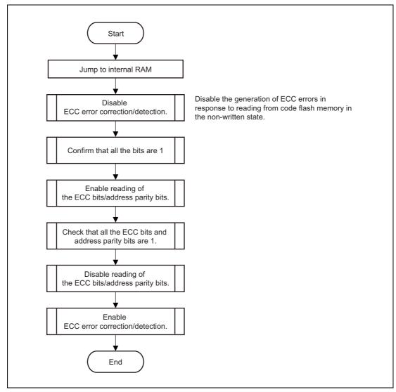
Figure 8.1 Blank Checking of Code Flash Memory
