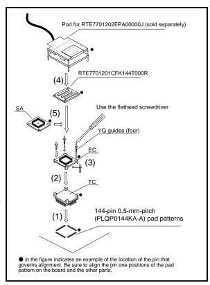
Figure 3 Procedure for Connecting the RTE7701201CFK144T000R
