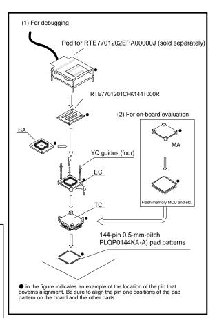
Figure 2 Usage of the RTE7701201CFK144T000R
