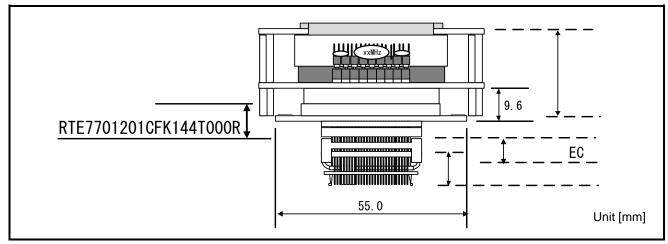
Figure 4 Drawing of the Socket Assembly
